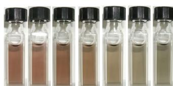
**Figure S4.** Photographs of 1.0 mg PEDOT-S in 4 mL of deionized water at various pH values of 9.2, 7.04, 6.00, 5.06, 3.52, 2.53 and 1.70 (from left to right) adjusted by the addition of 4  $\mu$ L of hydrazine followed by sequential additions of conc. HCl.
