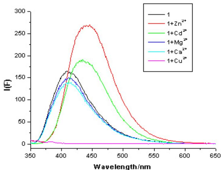
**Figure S8.** Fluorescence spectra of compound **1** ( $1.6 \mu\text{M}$ ,  $\lambda_{\text{ex}} = 340 \text{ nm}$ ) in an aqueous solution (20 mM HEPES, pH = 7.4, 125 mM NaCl, 1.2 mM  $\text{MgCl}_2$ , 5.9 mM KCl, 2.4 mM  $\text{CaCl}_2$ , 0.5 mM EDTA, and 0.5 mM EGTA) in the presence of 2.6 mM of  $\text{Zn}^{2+}$  (red),  $\text{Cd}^{2+}$  (green),  $\text{Mg}^{2+}$  (blue),  $\text{Ca}^{2+}$  (cyan), and  $\text{Cu}^{2+}$  (pink).
