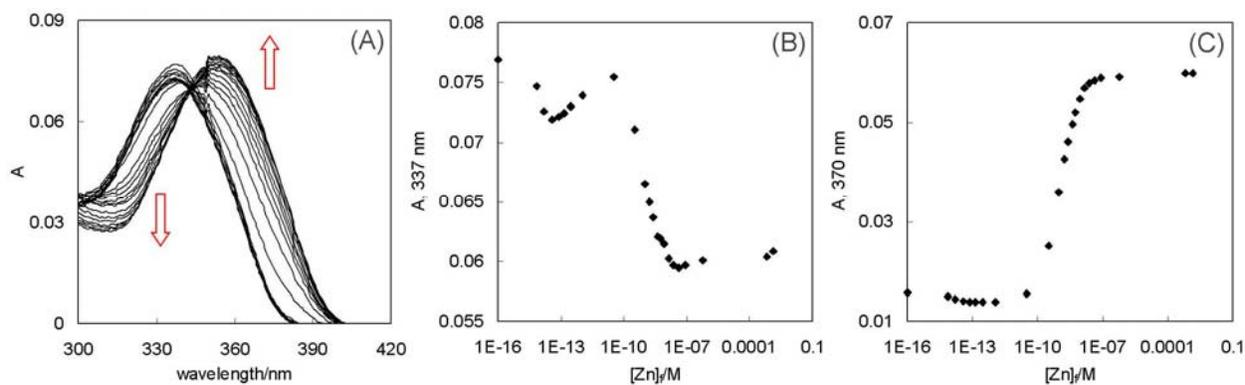
**Figure S5.** (A) Absorption spectra of **1** (2.0  $\mu\text{M}$ ) in the presence of  $\text{Zn}(\text{ClO}_4)_2$  (0 – 15.6 mM) in 10% DMSO aqueous solution (HEPES: 50 mM, pH = 7.0,  $\text{KNO}_3$ : 100 mM; EDTA: 5 mM; EGTA: 5 mM; NTA: 5 mM). Arrows represent the direction of spectral changes upon addition of zinc. Absorbance values of **1** at (B) 337 nm and at (C) 370 nm vs. the concentration of free zinc ion.
