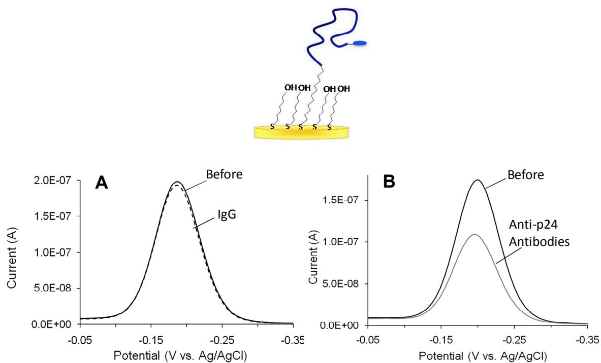
**S.I. 3** E-PB sensors fabricated with C6-OH as the diluent show similar selectivity as the C9-OH passivated sensors; however, sensor sensitivity appears to be adversely affected since less signal suppression is observed under the same experimental condition. Shown here are the sensors' responses in AC voltammetry when interrogated with (A) 43 nM IgG and (B) 43 nM anti-p24 antibodies in a Phys2 buffer. Conditions: AC frequency: 10 Hz; AC amplitude: 25 mV; incubation time: ~60 min.
