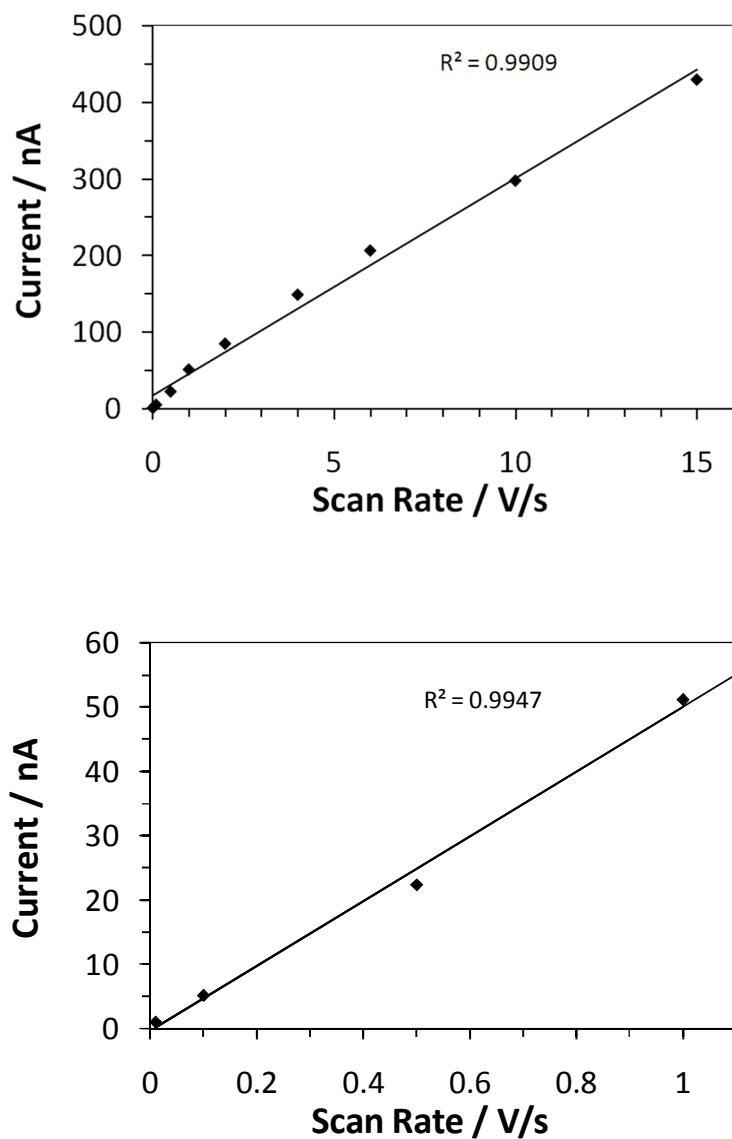
**S.I. 4** The linear relationship between peak currents and scan rates confirms that the redox species (MB) is confined to the electrode surface.
