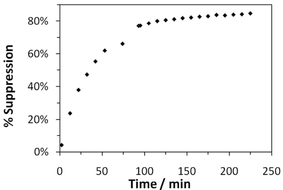
**S.I. 2** The E-PB sensor responses to its target in minutes. At a target antibody concentration of 43 nM, complete signal saturation time is  $\sim$ 100 min, but the majority of the response ( $>75\%$ ) is achieved within 60 min.
