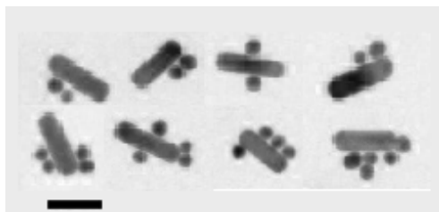
Fig. S1. Additional TEM images of AuNR-AuNPs junction showing the binding of AuNPs onto AuNRs through a thrombin sandwich assay (The scar bar is 50 nm).
