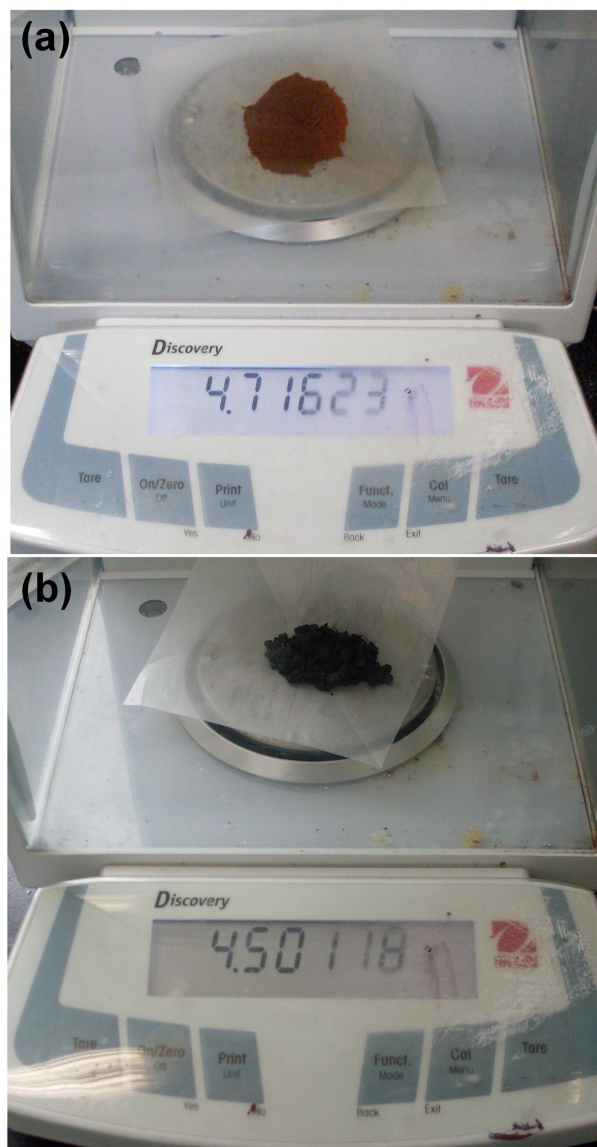
Figure S8. Photographs of (a) the \beta -FeOOH nanoparticles and (b) the final magnetite-C nanocomposite.
