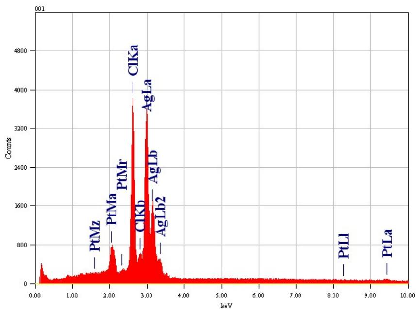
**Fig. S4.** EDS pattern of Pt/AgCl hetero-nanotubes.
