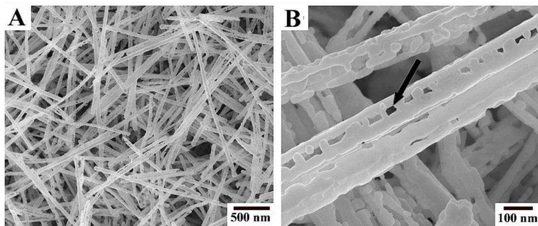
**Fig. S1.** (A, B) SEM images of AgCl hollow nanostructures.
