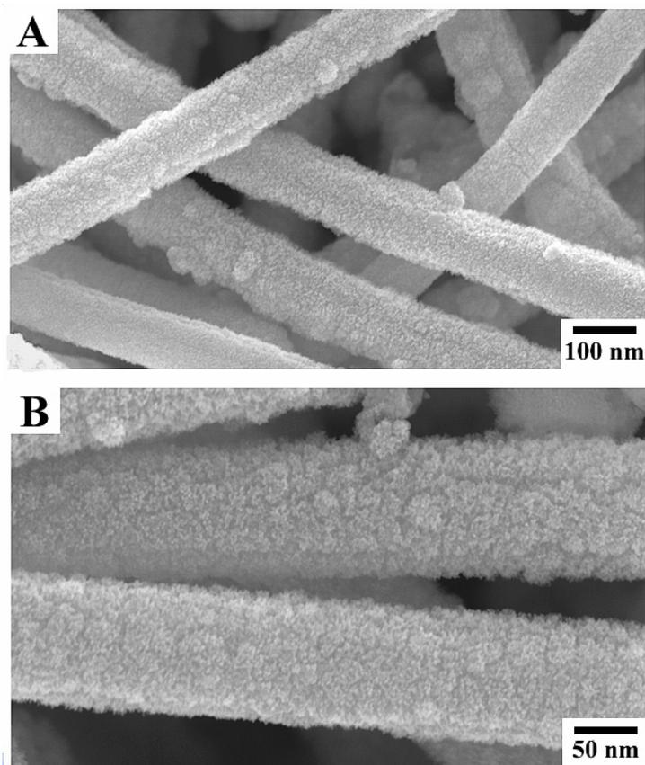
**Fig. S2.** (A,B) SEM images of Pt/AgCl hetero-nanotubes with different magnifications.
