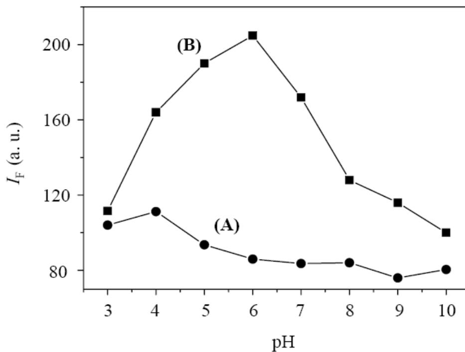
**Figure S2.** The effect of pH on the fluorescence intensity of DNA-Ag NCs in the (A) absence and (B) presence of  $\text{Cu}^{2+}$  ions (200 nM). DNA-Ag NCs were diluted with 20 mM phosphate solution to a final concentration of 0.004 X.
