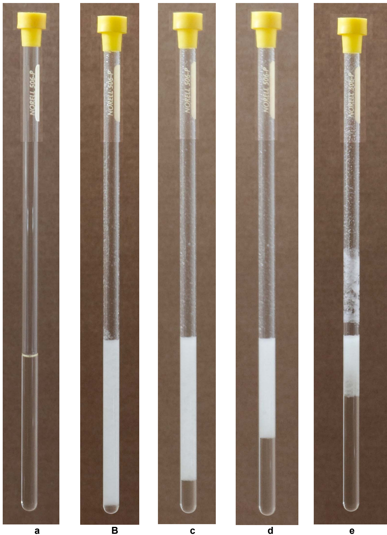
Figure S1. Pictures of the NMR tube: a – solution of 3 in CDCl 3 ; b – after addition of analyzed sample, DCC/DMAP and shaking for 1 min; c – after standing for 10 min; d – after standing for 20 min; e – after standing for 30 min.
