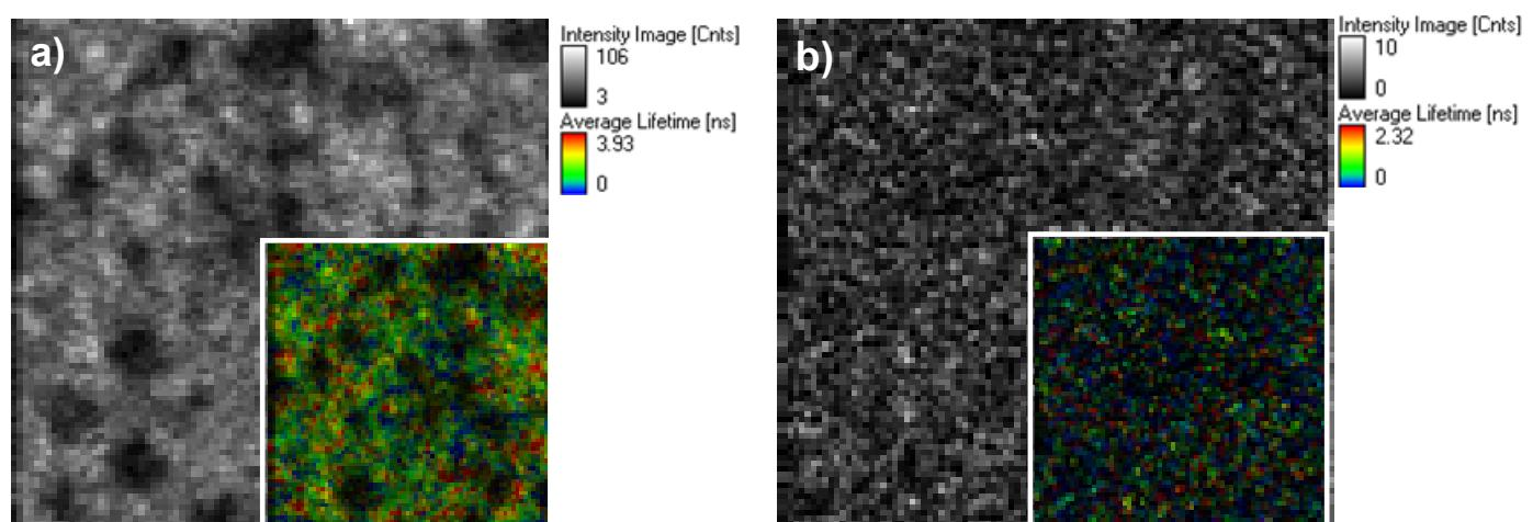
**Figure S2.** Intensity and lifetime fluorescence images ( $20 \times 20 \mu\text{m}$ ) of a) commercial cover glass (no cleaning, Roth) and b) the same cover glass modified with a monolayer of **2**. Below is presented the fluorescence lifetime histograms of the commercial cover glass (blue) and modified cover glass (pink).
