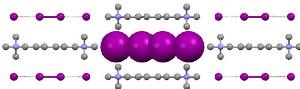
**Figure SI8.** The crystal packing of the complex **2** viewed down crystallographic  $c$  axis. Colour code: Carbon: gray, Nitrogen: pale blue, Iodine: purple. The hydrogen atoms are omitted for clarity. Central  $\text{I}_4^{-2}$  moiety is pictured in spacefill model.
