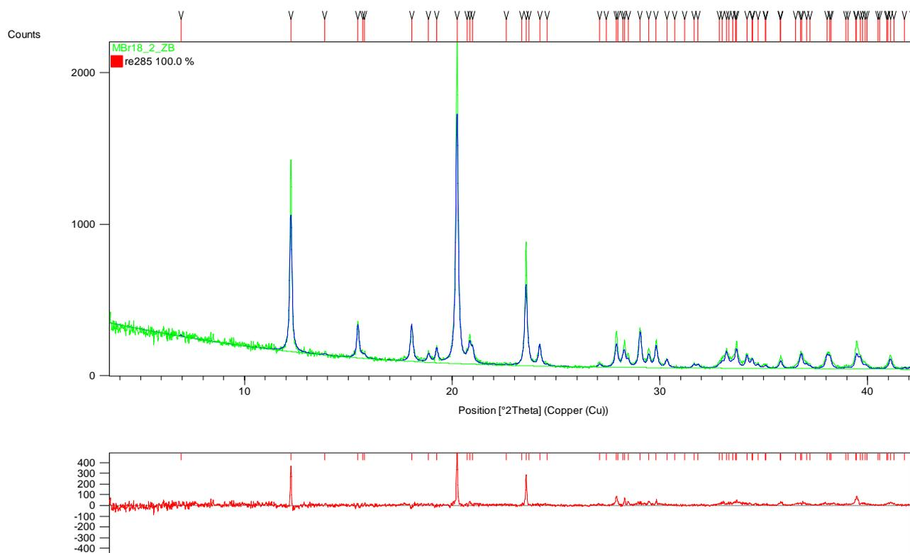
**Figure SI14.** Final Rietveld refinement plot of  $2_{\text{pwd3}}$ . The red tick marks on top represent the diffraction positions, green line the observed pattern, blue line the best fitted profile, and the red difference curve between observed and calculated profile at the lower graph.
