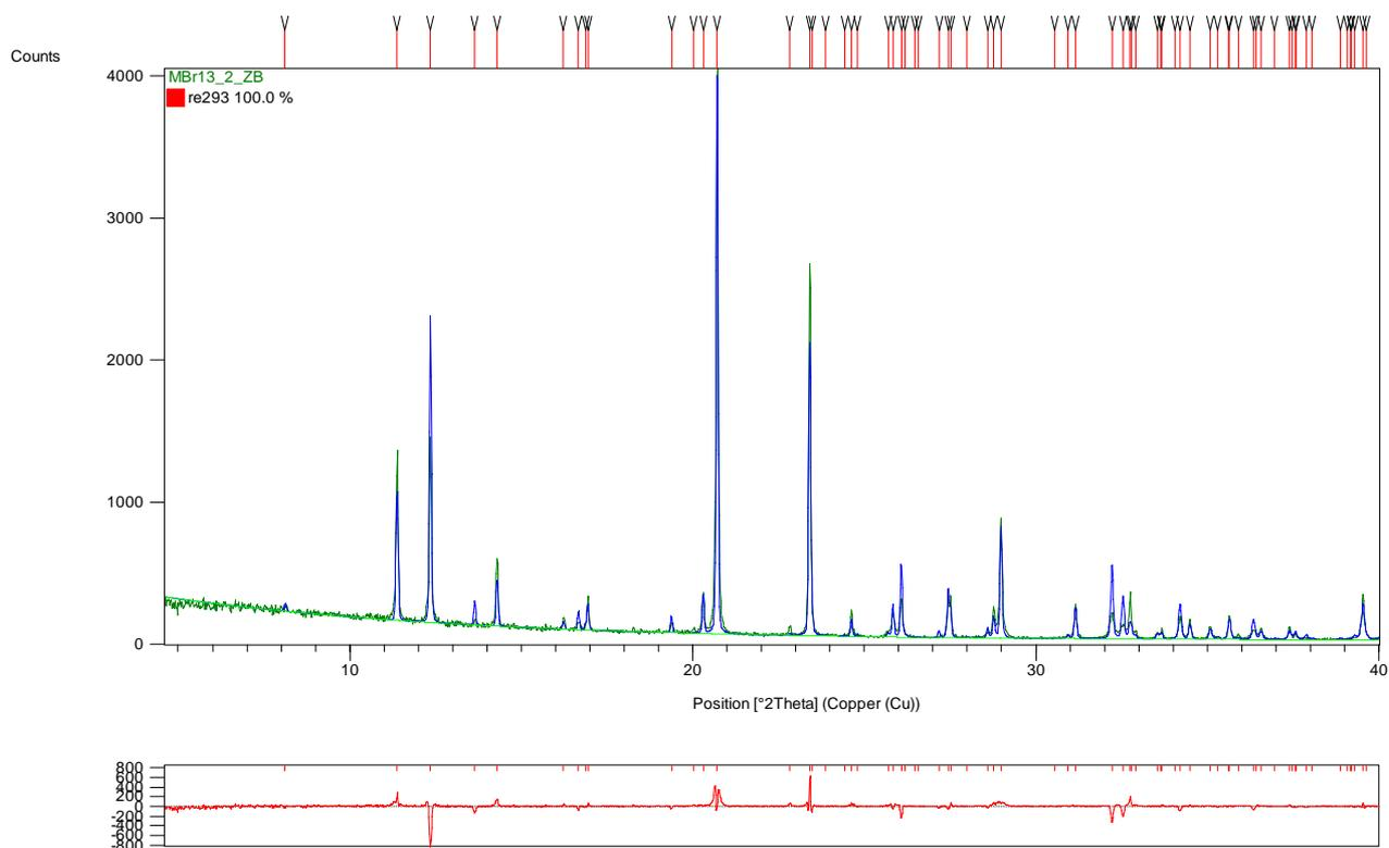
**Figure SI12.** Final Rietveld refinement plot of  $3_{\text{pwd1}}$ . The red tick marks on top represent the diffraction positions, green line the observed pattern, blue line the best fitted profile, and the red difference curve between observed and calculated profile at the lower graph.
