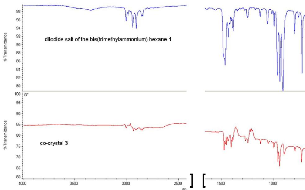
**Figure SI5.** IR spectra for **1** and co-crystal **3**
