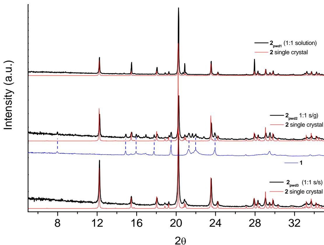
**Figure SI13.** XRD patterns of **1** (hexamethonium iodide),  $2_{\text{pwd1}}$  (1:1 solution),  $2_{\text{pwd2}}$  (1:1 solid/gas) and  $2_{\text{pwd3}}$  (1:1 solid/solid) compared to the simulated diffraction pattern of the expected single crystal structure  $2_{\text{sc}}$ . Some diffraction peaks of hexamethonium iodide impurity on  $2_{\text{pwd2}}$  pattern is pointed out by dashed blue lines.
