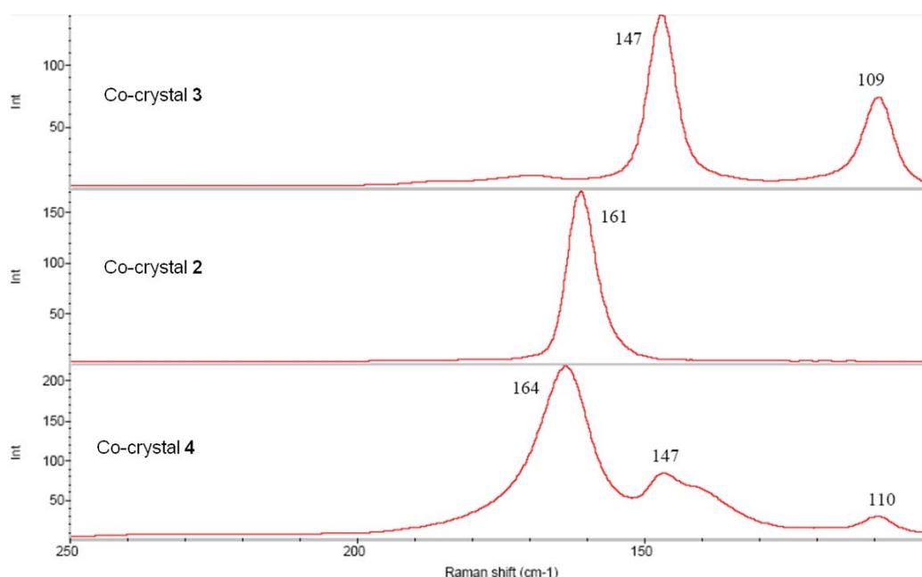
**Figure SI7.** Raman spectra for the co-crystals **2**, **3** and **4**
