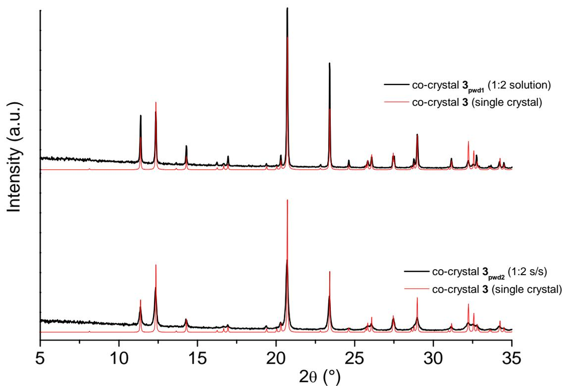
**Figure SI11.** XRD patterns of  $3_{\text{pwd1}}$  (1:2 solution) and  $3_{\text{pwd2}}$  (1:2 solid/solid reaction) compared to the simulated XRD pattern of expected single crystal structure  $3_{\text{sc}}$ .
