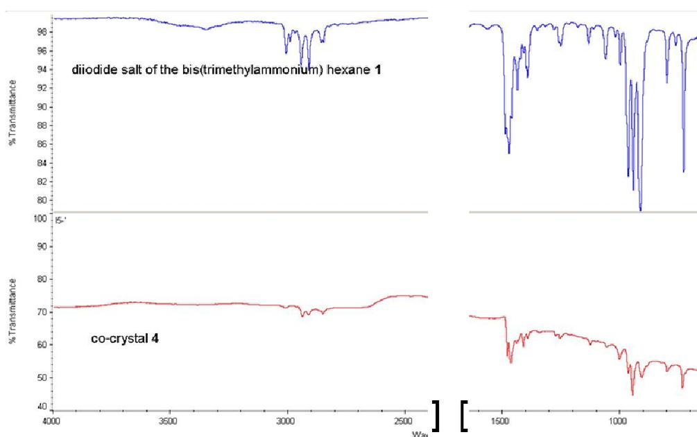
**Figure SI6.** IR spectra for **1** and co-crystal **4**
