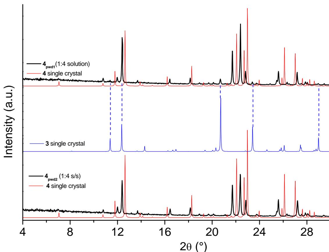
**Figure SI15.** XRD patterns of  $4_{\text{pwd1}}$  (1:4 solution) and  $4_{\text{pwd2}}$  (1:4 solid/solid) compared to simulated patterns of two single crystal structures (**4** and **3**). The peak positions of  $3_{\text{sc}}$  phase in  $4_{\text{pwd1}}$  pattern is pointed out by dashed blue lines.
