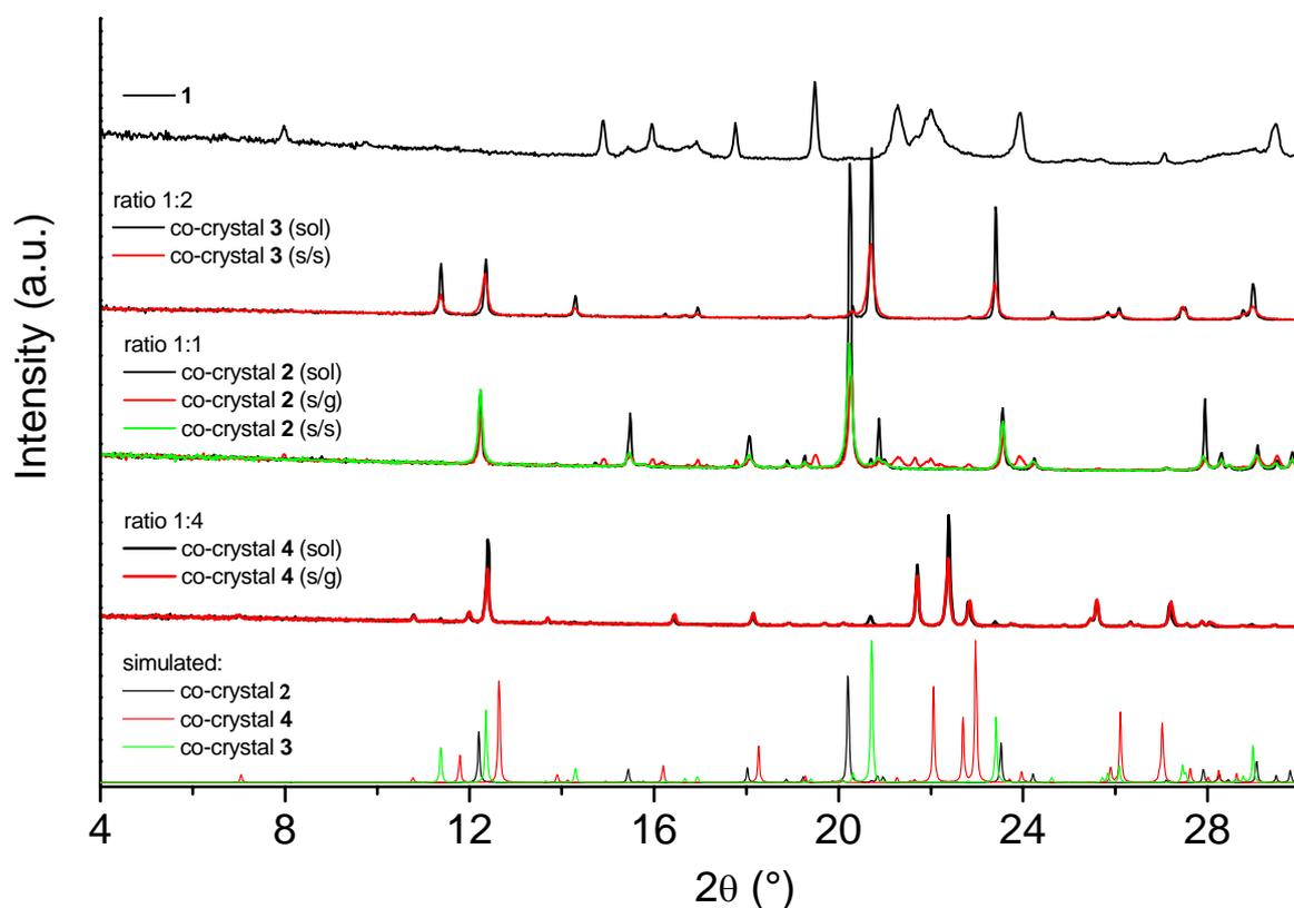
**Figure SI10.** XRD patterns of compound **1** and co-crystal **2**, **3** and **4**, and the simulated patterns of single crystal structure. Patterns are grouped by the mixing ratio of hexamethonium iodide and iodine. (sol: solution; s/s: solid/solid; s/g: solid/gas)
