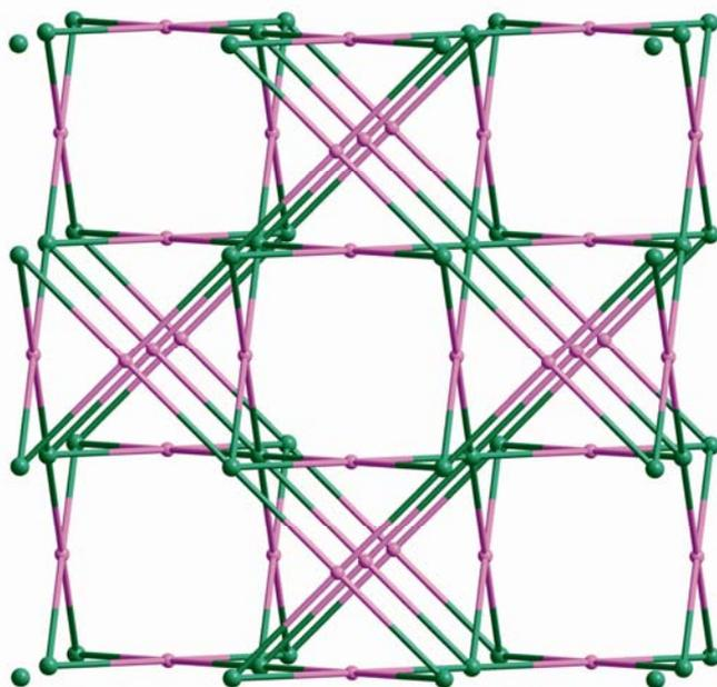
**Fig. S2** The schematic representation of the complicated connectivity between clusters in the Cu-S framework. The balls represent [Cu<sub>8</sub>S<sub>12</sub>]<sup>16-</sup> (green) and [Cu<sub>8</sub>S<sub>16</sub>]<sup>24-</sup> (pink) clusters, which are in hexagonal and tetragonal coordination environment, respectively.
