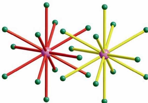
**Fig. S4** Schematic representation of the two interpenetrating channel systems along  $\langle 110 \rangle$  in **1**.
