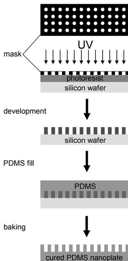
Figure 1. Fabrication of nanoplates. A photomask is generated using a computer animated design (CAD) program. Subsequently the pattern is projected onto a silicon wafer coated with photoresist using UV light. Specific polymerization of the exposed areas results in a mold that can be filled with PDMS. After baking, the cured PDMS is peeled off and can optionally be rendered hydrophilic by plasma treatment.
