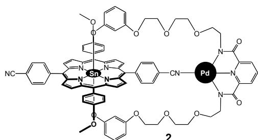
In a dry 50 mL two-necked round-bottom flask, compound **21** (23 mg, 0.03 mmol, 1 eq.) was introduced. A solution of palladium complex **15** (20 mg, 0.03 mmol, 1 eq.) in 15 mL of CH<sub>2</sub>Cl<sub>2</sub> was added under argon. The reaction mixture was stirred at room temperature under argon for 2 days. The solvent was evaporated to dryness and the residue was crystallised from a toluene/pentane mixture (1/2, 45 mL) to yield the desired complex **2** (34 mg, 83%) as a green solid.
