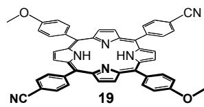
In a 250 mL two-necked round-bottom flask, compound **18** (2.0 g, 8.1 mmol, 1 eq.) was dissolved in 150 mL of a CH<sub>2</sub>Cl<sub>2</sub>/EtOH mixture (95/5). To the solution, compound **17** (1.0 mL, 8.2 mmol, 1 eq.) was added and the mixture was degassed using argon for 5 min. Under argon and in exclusion of light, TFA (1.2 mL, 16.2 mmol, 2 eq.) was added and the solution
