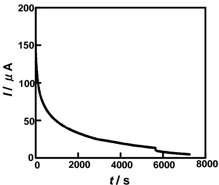
**Fig. S2.** An Amperometric *i-t* curve for glucose oxidation by Rh(DPDE)/C. The potential was maintained at  $-0.5$  V (vs. Ag|AgCl|KCl(sat.)). The electrolyte solution (15 mL, 1 M NaOH) containing 10 mM glucose was purged with argon gas, and anaerobic conditions were maintained by purging with argon gas during electrolysis. The electrolyte solution was stirred using a magnetic stirrer.
