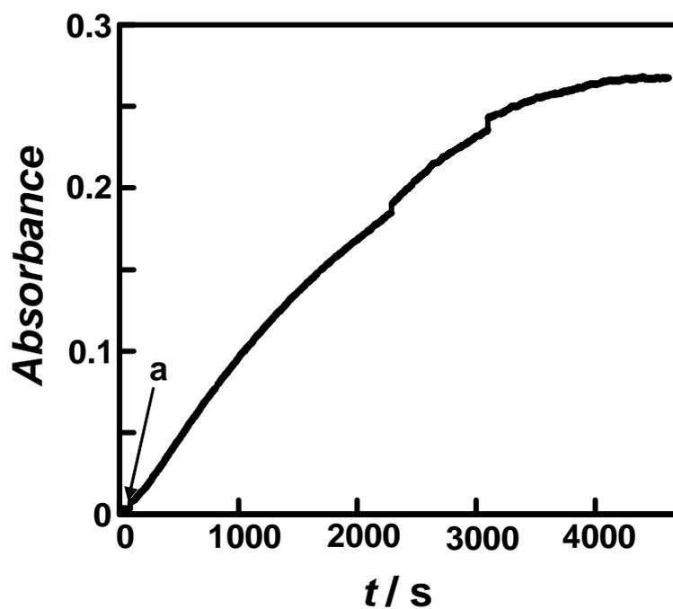
**Fig. S3.** A profile of absorbance at 340 nm of the solution after electrolysis. The solution contains  $\text{NADP}^+$  (0.96 mM), 6-PGDH, ATP (3.6 mM), and  $\text{MgCl}_2$  (1.0 mM). The solution of GK was added at arrow *a*. The increase in the absorbance corresponds to the amount of gluconate.
