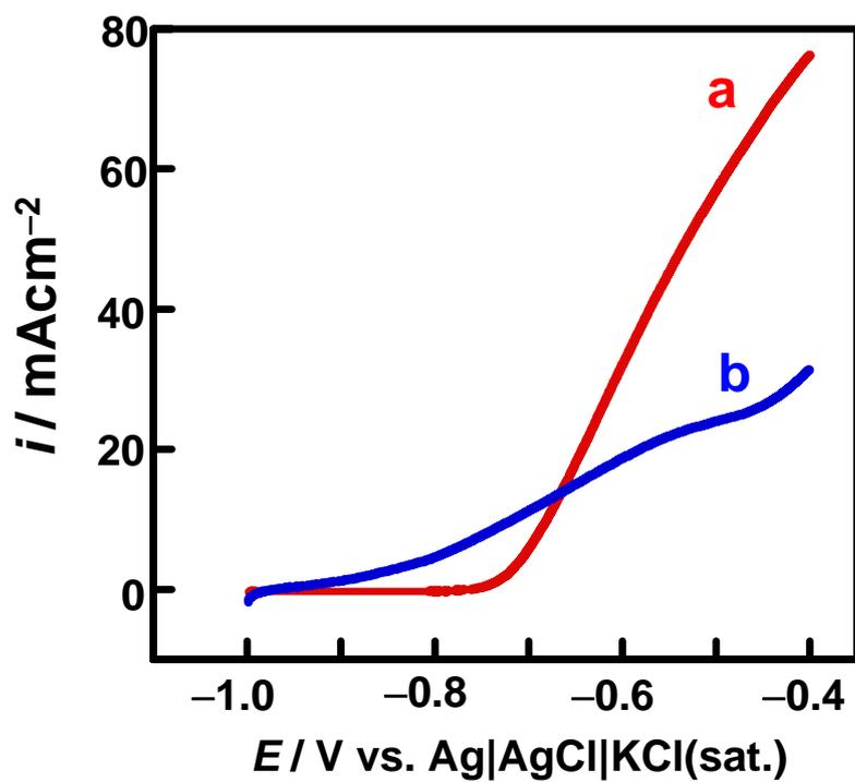
**Fig. S1.** Voltammograms of (a) Rh(DPDE)/C and (b) Pt/C in the presence of 0.5 M glucose with electrode rotation at 6400 rpm (scan rate = 10 mV/s). The measurements were performed in 1 M NaOH under a  $\text{N}_2$  atmosphere.
