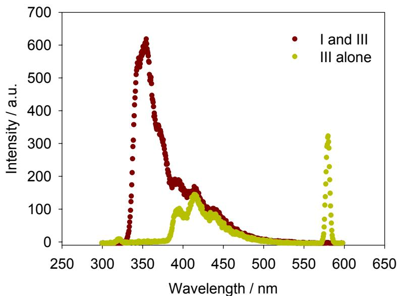
**Figure S7.** Emission spectra for solutions of III (0.060 mM) and a solution of I (2.2 mM) containing III (0.060 mM) at high pH. The sharp peak at 560 nm is due to Rayleigh scatter arising from poor excitation of III at this excitation.
