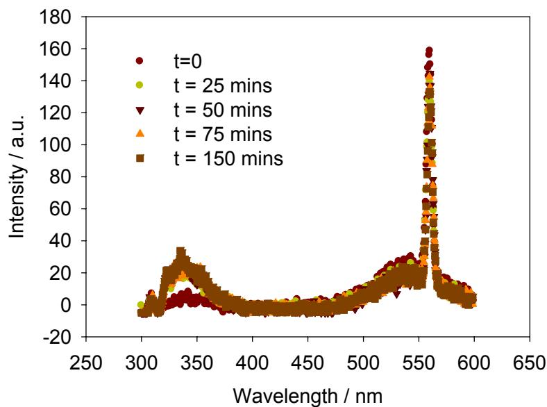
**Figure S4.** Evolution in emission from II alone (0.084 mM, excitation wavelength = 280 nm) on addition of GdL (3.75 mg/mL). As can be seen, no significant change in the emission is observed from II alone as the pH decreases. The sharp peak at 560 nm is due to Rayleigh scatter arising from poor excitation of II at this excitation.
