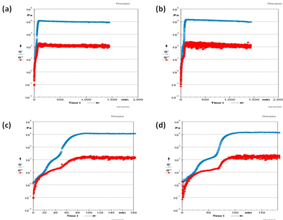
**Figure S2.** (a) Evolution of  $G'$  and  $G''$  with time for a solution of dipeptide I (2.2 mM) on addition of GdL (3.75 mg/mL). (b) Evolution of  $G'$  and  $G''$  with time for a solution of dipeptide I (2.2 mM) containing II (0.17 mM) on addition of GdL (3.75 mg/mL). (c) Expansion of (a) showing first 180 minutes. (d) Expansion of (b) showing first 180 minutes. In all cases, the blue data represents  $G'$  and red data  $G''$ .
