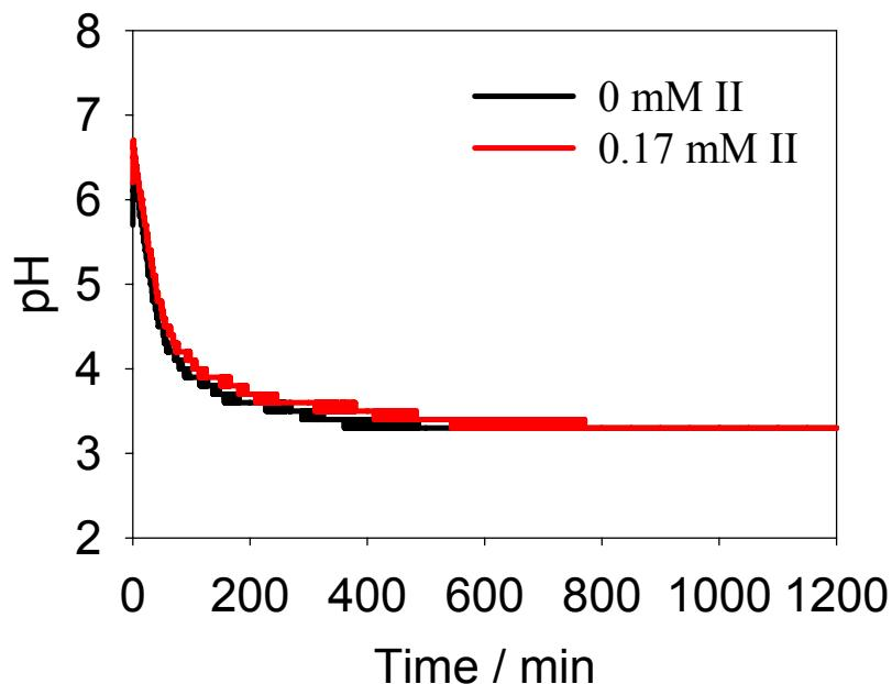
**Figure S1.** (Black data) Evolution of pH with time for a solution of dipeptide I (2.2 mM) on addition of GdL (3.75 mg/mL). (Red data) Evolution of pH with time for a solution of dipeptide I (2.2 mM) containing II (0.17 mM) on addition of GdL (3.75 mg/mL).
