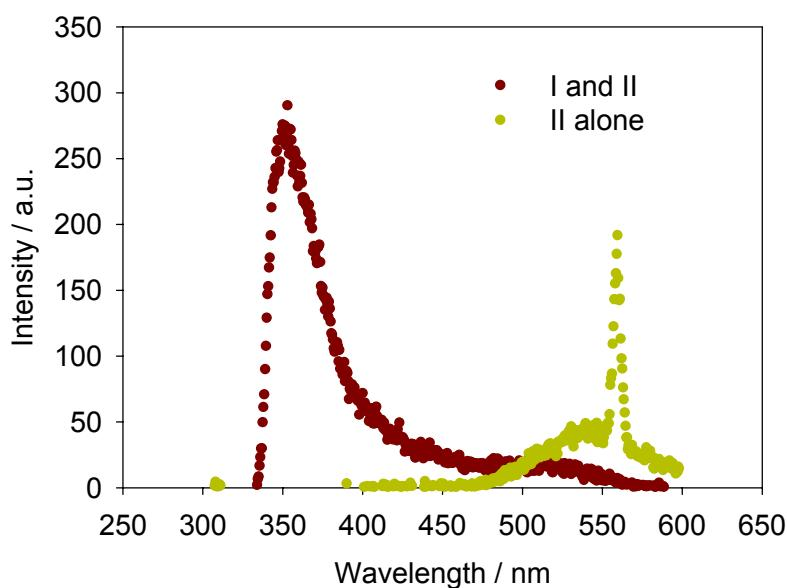
**Figure S6.** Emission spectra for solutions of II (0.164 mM) and a solution of I (2.2 mM) with added II (0.164 mM) at high pH. The sharp peak at 580 nm is due to Rayleigh scatter arising from poor excitation of II at this excitation.
