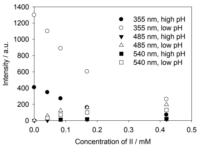
**Figure S8.** Variation in emission intensity at 355, 485 and 540 nm on addition of GdL (3.75 mg/mL) to a solution of I (2.2 mM) with added II. Without II, the intensity at 355 nm increases as gelation occurs. The increase is less apparent at low concentrations of II and decreases significantly at the higher concentrations of II. In all cases, the intensity at 485 nm
