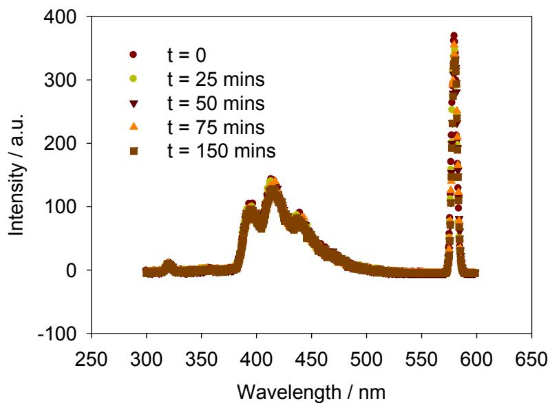
**Figure S5.** Evolution in emission from III (0.060 mM, excitation wavelength = 290 nm) alone on addition of GdL (3.75 mg/mL). As can be seen, no significant change in the emission is observed from III alone as the pH decreases. The sharp peak at 580 nm is due to Rayleigh scatter arising from poor excitation of III at this excitation.
