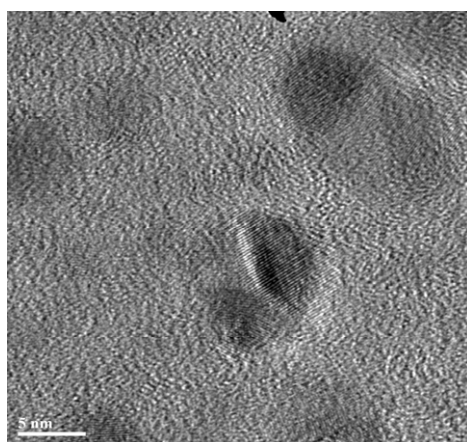
Supplementary Fig. 2 High resolution transmission electron microscopy of Cu nanocrystals.
