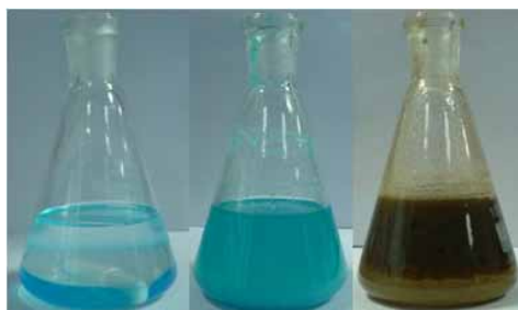
Supplementary Fig. 5 Photographs of large-scale syntheses of hydrophobic Cu nanocrystals in toluene-water system.
