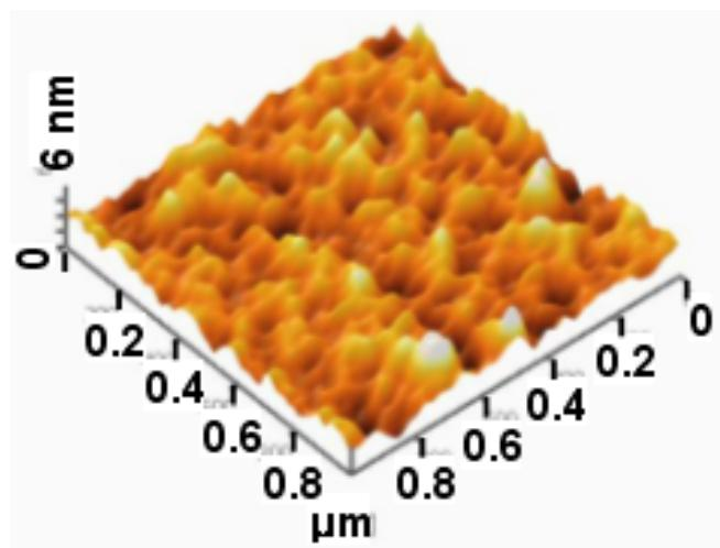
Figure S2. AFM image of PEDOT thin film with a root mean square surface roughness of 1 nm.
