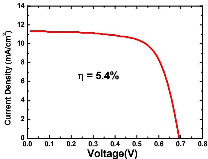
Figure S4. Current density-voltage characteristics of DSSCs with PEDOT/FTO counter electrode (800  $\text{S}/\text{cm}^2$ )
