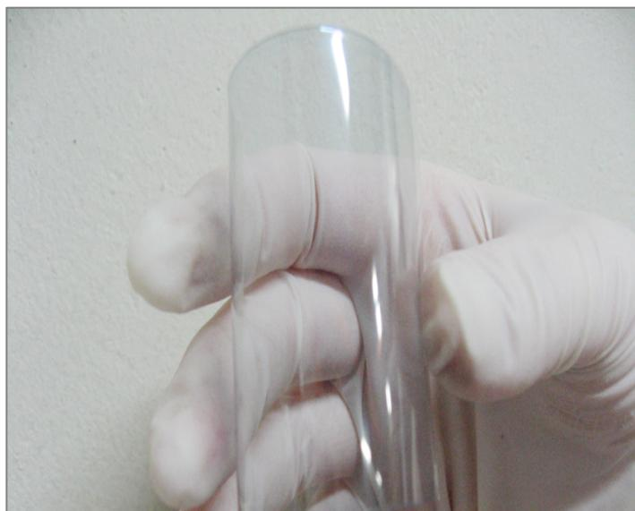
Figure S1. PEDOT thin film with a thickness of approximately 60 nm on PET substrate with surface resistivity of  $130 \Omega/\square$  and 88% transmittance at 550 nm.
