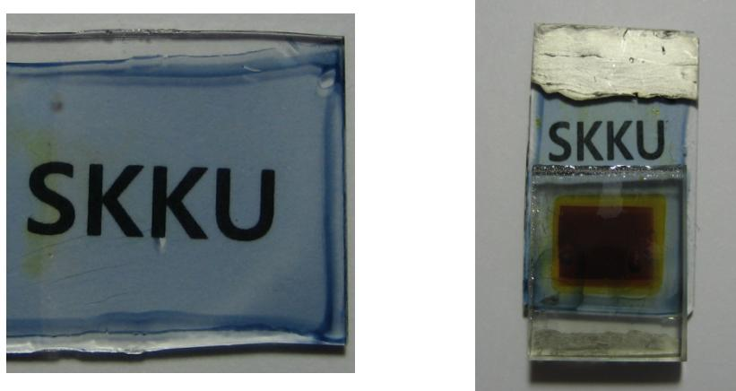
Figure S3. PEDOT thin film on glass substrate with 800 S/cm conductivity (left) and photograph of DSSC with Pt- and TCO- free counter electrode.
