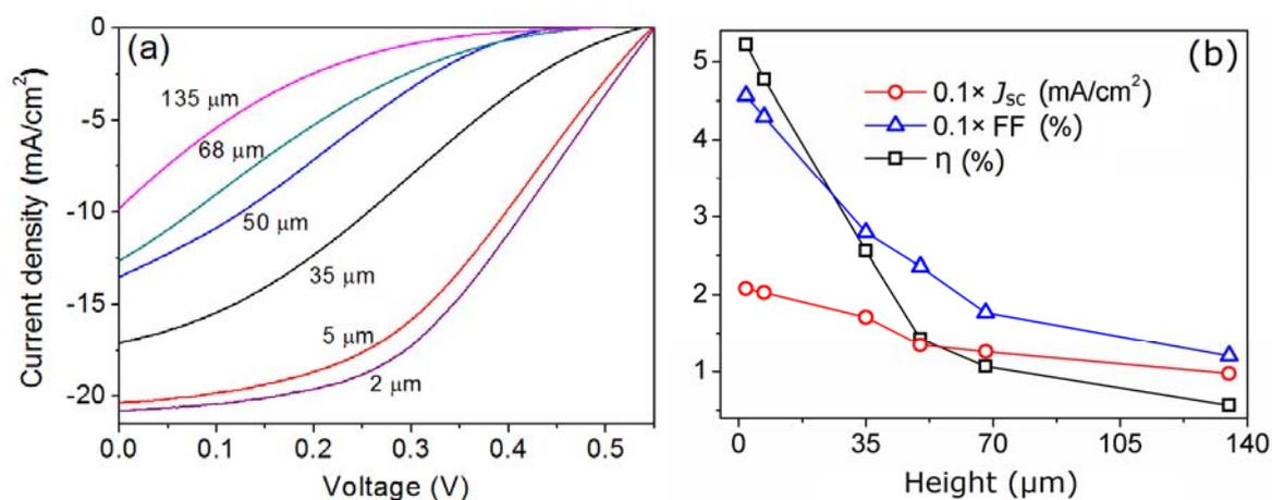
**Fig. S3** (a) Light  $J$ - $V$  curves of the hybrid solar cells made from SiNW arrays of different height. (b) Plots of  $J_{sc}$ , FF and  $\eta$  as a function of the array height. The transmittance at 550 nm of the CNT film is  $\sim 75\%$ .
