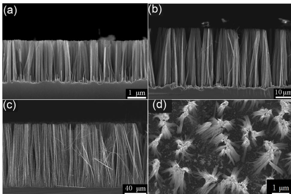
**Fig. S2** SEM images of the SiNW arrays. (a) Height=2 μm. (b) Height=35 μm. (c) Height=135 μm. (d) Top view.
