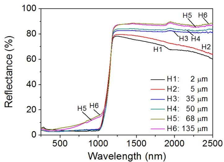
**Fig. S4** Reflection spectra of SiNW arrays of different height.
