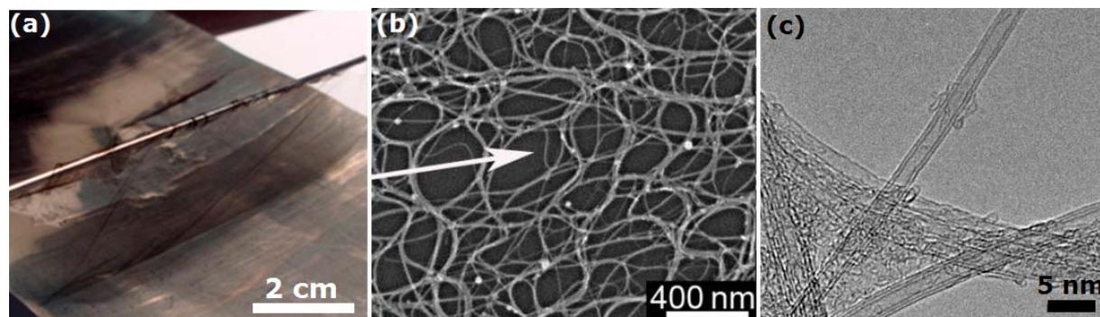
**Fig. S1** (a) Photograph of a freestanding CNT film being peeled off the nickel foil. (b) SEM image. (c) TEM image.
