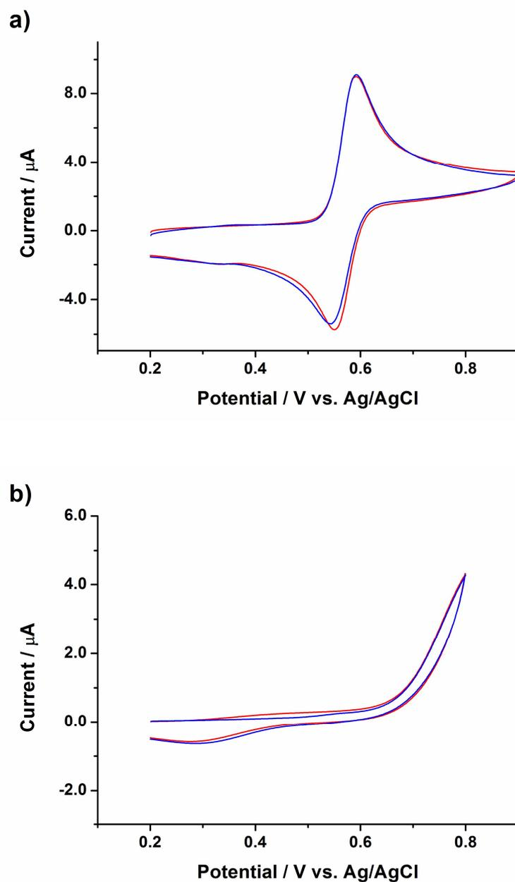
**Fig. S2** Cyclic voltammograms for DOPA on a) bare gold and b) BDT-modified gold electrodes in 0.25 M  $\text{H}_2\text{SO}_4$  (pH 0.6). The scan rate was 50 mV/s. The electrode area was  $2.01 \text{ mm}^2$ . The red and blue curves indicate the voltammograms for D- and L-DOPA, respectively.
