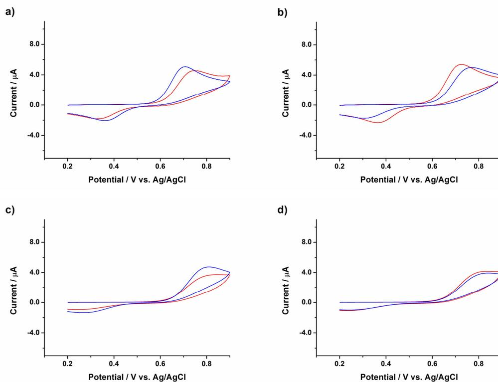
**Fig. S6** Cyclic voltammograms for enantioselective recognition of DOPA using Pen-AuNPs of various sizes in 0.25 M  $\text{H}_2\text{SO}_4$  (pH 0.6). The scan rate was 50 mV/s. The electrode area was  $2.01 \text{ mm}^2$ . a) 3.1-nm-diameter D-Pen AuNPs, b) 3.1-nm-diameter L-Pen-AuNPs, c) 4.0-nm-diameter D-Pen AuNPs, and d) 4.0-nm-diameter L-Pen-AuNP-immobilized gold electrodes. The red and blue curves indicate the voltammograms for D- and L-DOPA, respectively.
