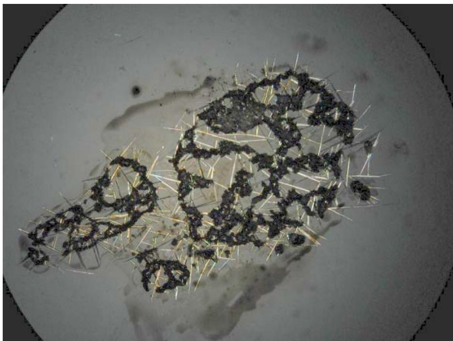
Figure S2. Sublimation of (*S,S*)-10. View of the fine needles of (*S,S*)-10 through crossed-polarizers on the hot-stage microscope.
