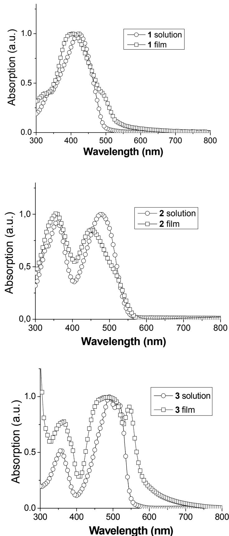
**Figure S3.** Optical density of **1-3** in dichloromethane and as spin-coated film on quartz.
