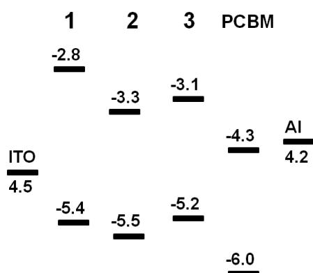
**Figure S5.** Experimental values obtained for the energy levels of **1-3** and PCBM.
