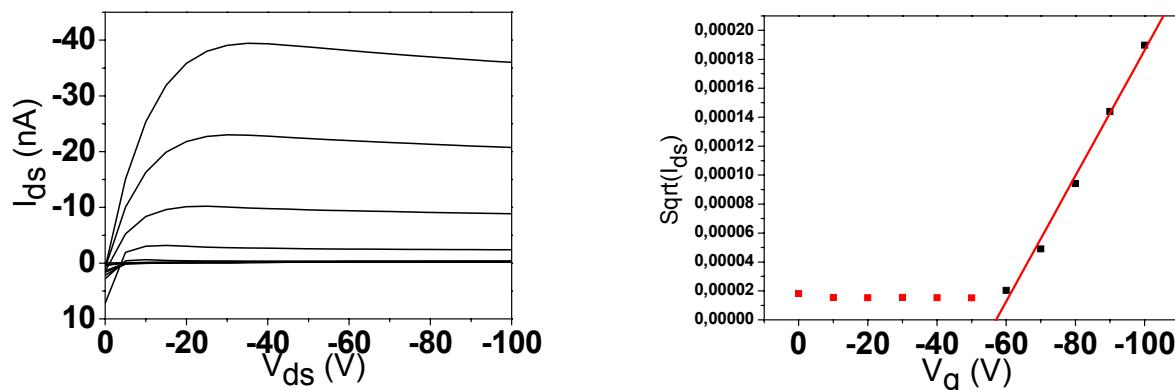
**Figure S6.** OTFT  $I_{ds}$  vs.  $V_{ds}$  current – voltage characteristics and square-root of  $I_{ds}$  vs. gate bias for compounds **3**. The extracted field effect mobility is  $\mu = 2.09 * 10^{-4} \text{ cm}^2/\text{V}\cdot\text{s}$ , the threshold voltage is  $V_t = 57.07 \text{ V}$  while the on/off ratio is 109.56
