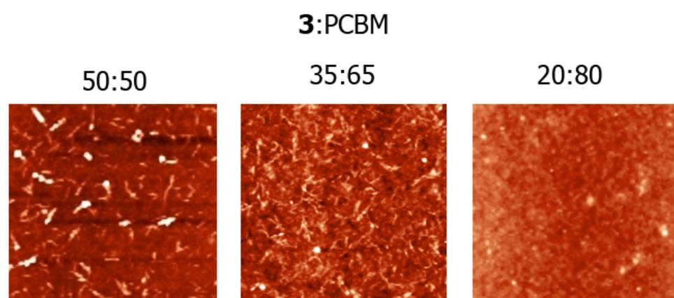
**Figure S7.** Tapping mode AFM topography images ( $10 \mu\text{m} \times 10 \mu\text{m}$ ) of **3:PCBM** at different PCBM concentrations.
