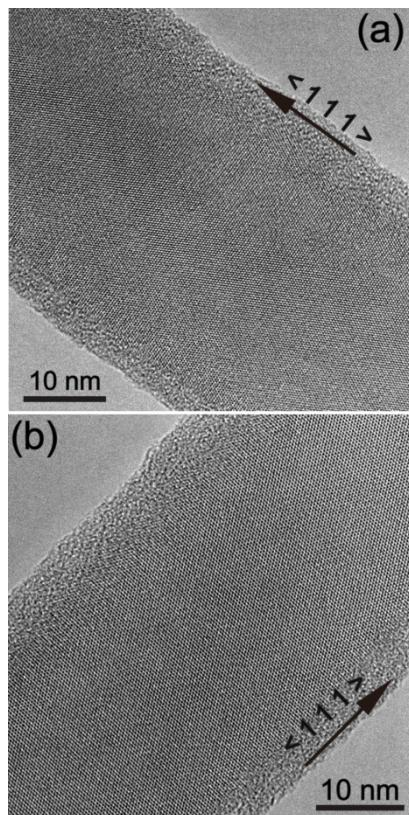
Figure S5. HRTEM images of two SiNWs with a diameter of (a) 38,(b) 41 nm, respectively.
