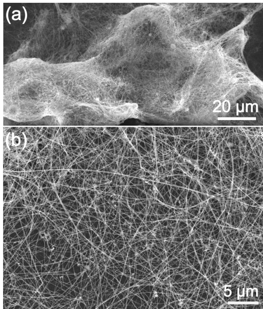
Figure S4. SEM image of Si nanowire synthesized by thermal decomposition of MPS in anhydrous toluene at 480°C by LICVD
