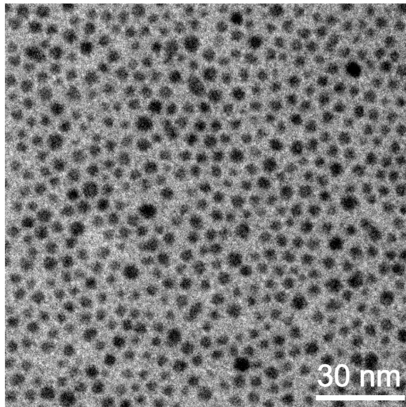
Figure S1. TEM image of dodecanethiol-coated Au nanocrystals.
