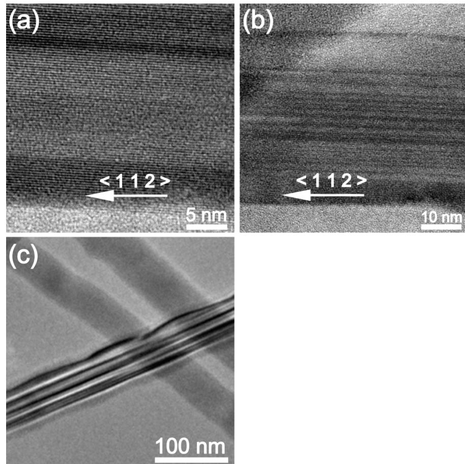
Figure. S6 TEM images of Si nanowires with  $\langle 112 \rangle$  growth directions. These nanowires were grown by LICVD with Au nanocrystals. The nanowires have multiple  $\{111\}$  twins extending down their length oriented parallel to their  $\langle 112 \rangle$  growth direction.
