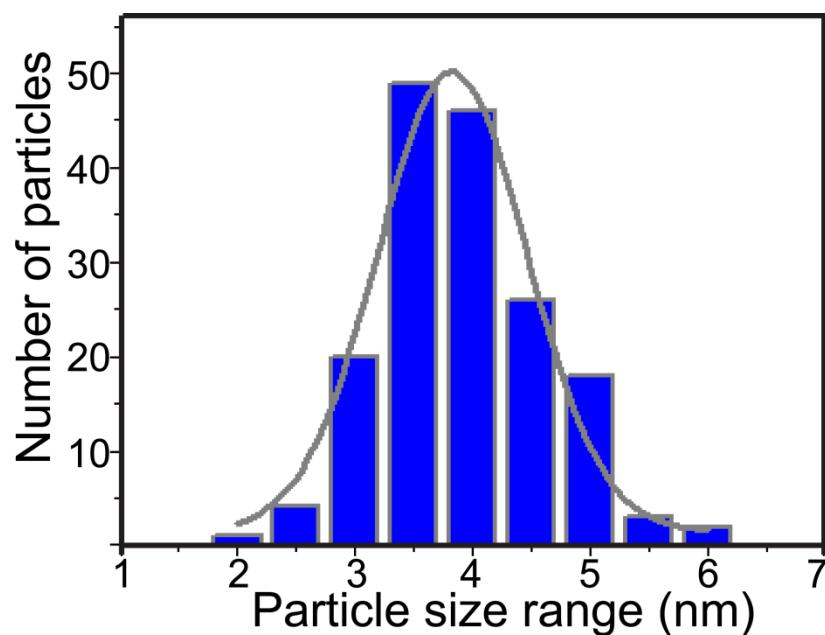
Figure S2. The size distribution of Au nanocrystals. The smooth curves show a Gaussian fit of the nanocrystals distributions.
