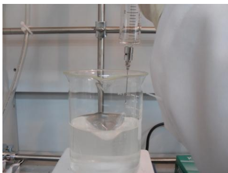
Figure S1. Photo image of fabrication of single O/W emulsion.
