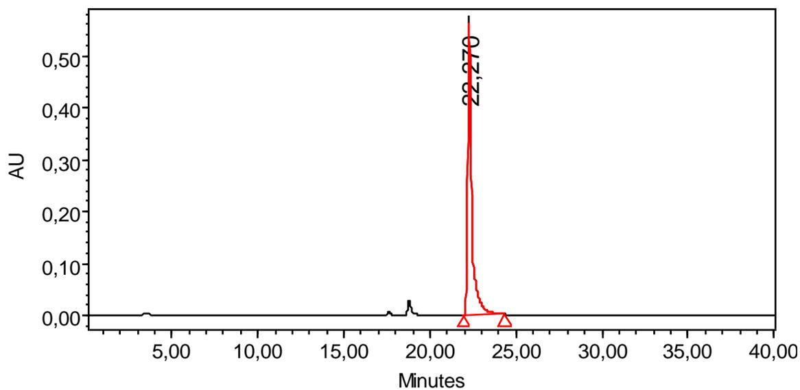
**Figure S15.** HPLC trace at 254 nm of purified compound **9**.
