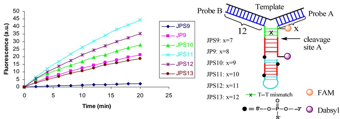
**Figure S4.** The base-pairing numbers between template and probes A (designated as x) influence the cleavage of JP tripartite by BfuCI. [Probes A] = [probe B] = 200 nM, [DNA template] = 1 nM, [BfuCI] = 0.1 U/ $\mu$ L, assay temperature = 35  $^{\circ}$ C.  $\lambda_{\text{ex}}$  = 494 nm,  $\lambda_{\text{em}}$  = 522 nm, slit<sub>ex</sub> = slit<sub>em</sub> = 10 nm, PMT = 600 V.
