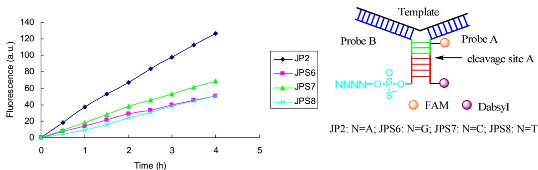
**Figure S3.** All probes are modified at site B with phosphorothioate. The sequence contents of the probe B 5'-overhangs are however different. [Probes A] = [probe B] = 1  $\mu$ M, [DNA template] = 0.2  $\mu$ M, [BfuCI] = 0.033 U/ $\mu$ L. Fluorescence data is normalized.  $\lambda_{\text{ex}}$  = 494 nm,  $\lambda_{\text{em}}$  = 522 nm, slit<sub>ex</sub> = slit<sub>em</sub> = 5 nm, PMT = 600 V.
