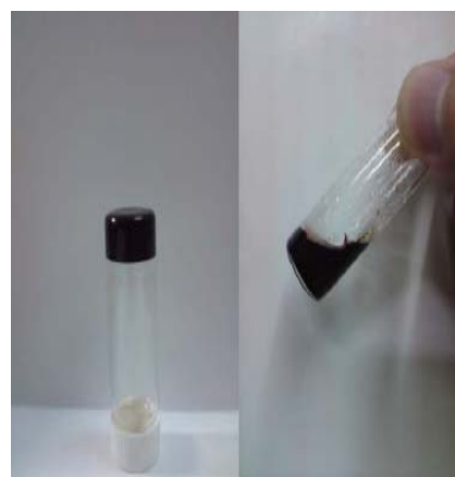
Fig. S9. Optical micrograph of inverted vials 20-30 min at room temperature after vial inversion with (left) the elastic gel SPI-U/SMA-A and (right) the crosslinking SPI-U/SMA-A fluid after heating at 80 °C. All polymers and additives were dissolved in m-cresol.
