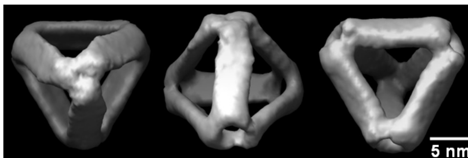
Figure S3. Three views of the DNA tetrahedron with hairpin structures reconstructed by relaxing to lower C3 symmetry.
