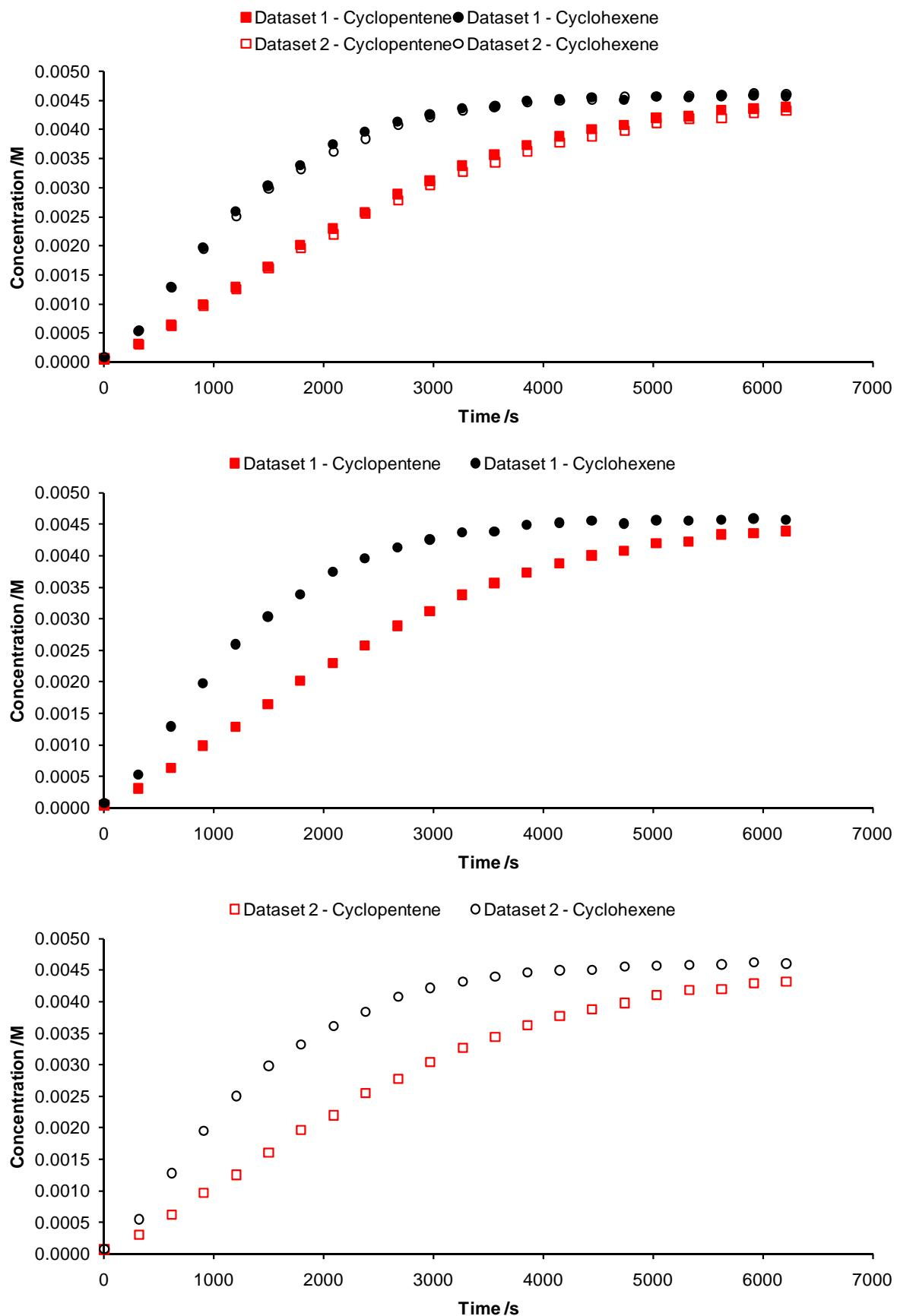
*Concentration/time data for the RCM of heptadiene 7b and octadiene 7c with pre-catalyst 9 in CDCl<sub>3</sub> at 298 K (AV400, BBFO-z-ATMA probe); 4 scans with D<sub>I</sub> = 35 s; TE = 298 K; concentrations obtained by integration of the appropriate signal and the internal standard (see above), with the exception of heptadiene which was calculated from [diene]-[octadiene].*
