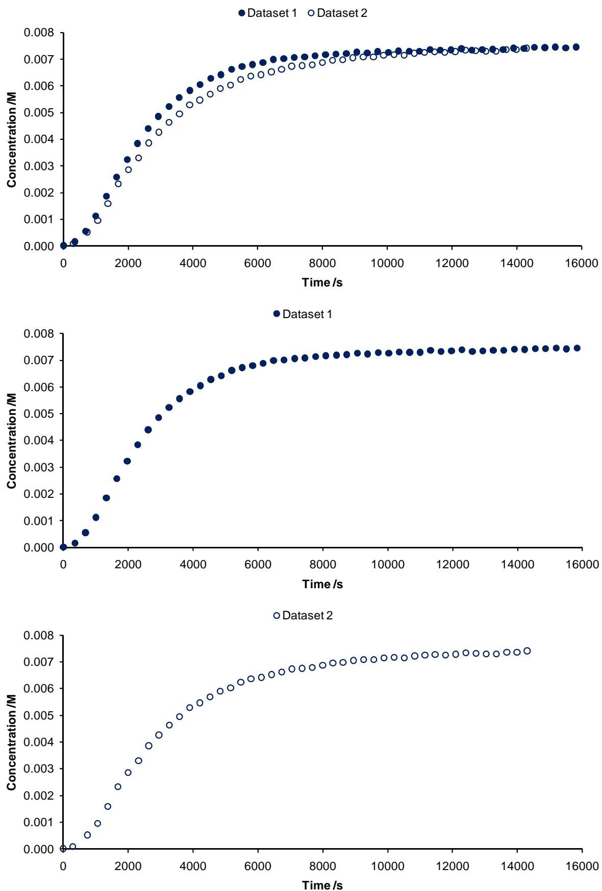
*Concentration/time data for the RCM of nonadiene **7d** with pre-catalyst **9** in CDCl<sub>3</sub> at 298 K (AV600, BBO-z-ATMA probe); 4 scans with D<sub>I</sub> = 35 s; TE = 298 K; concentrations obtained by integration of the appropriate signal and the internal standard (see above).*
