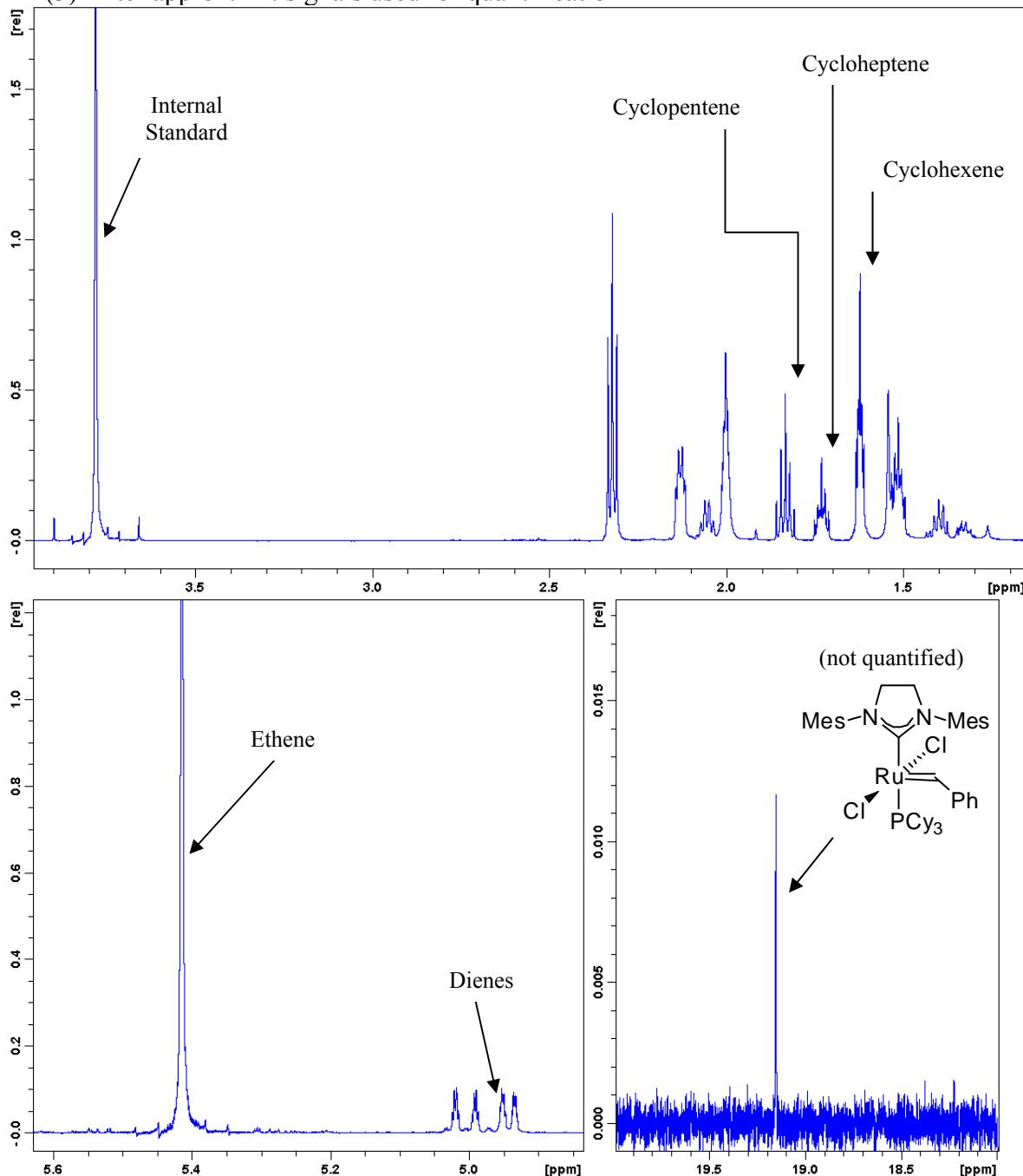
*Concentration/time data for the RCM of heptadiene 7b, octadiene 7c, nonadiene 7d with pre-catalyst 9 in CDCl<sub>3</sub> at 298 K (AV600, TBI-z probe); 4 scans with D<sub>1</sub> = 35 s; TE = 298 K; concentrations obtained by integration of the appropriate signal and the internal standard (see above).*
