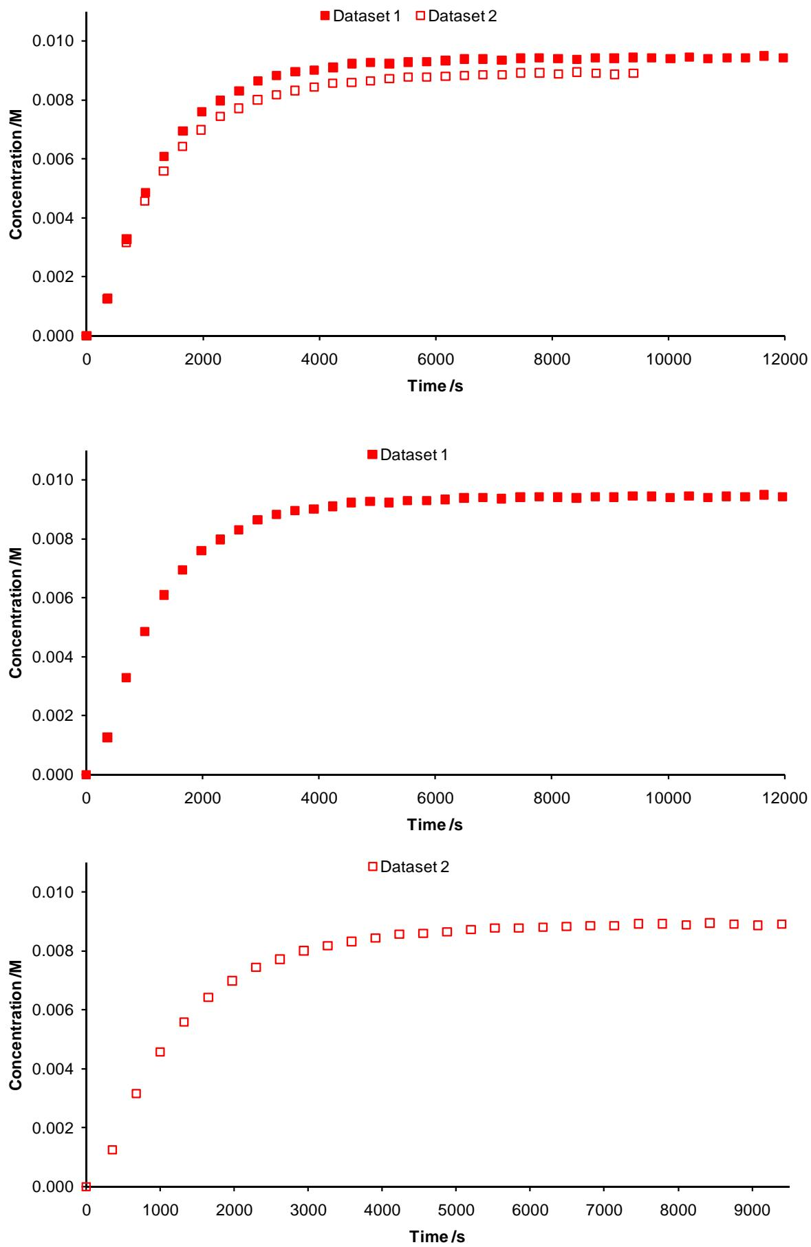
*Concentration/time data for the RCM of heptadiene 7b with pre-catalyst 9 in CD<sub>2</sub>Cl<sub>2</sub> at 298 K (AV600, BBO-z-ATMA probe); 4 scans with D<sub>1</sub> = 35 s; TE = 298 K; concentrations obtained by integration of the appropriate signal and the internal standard (see above).*
