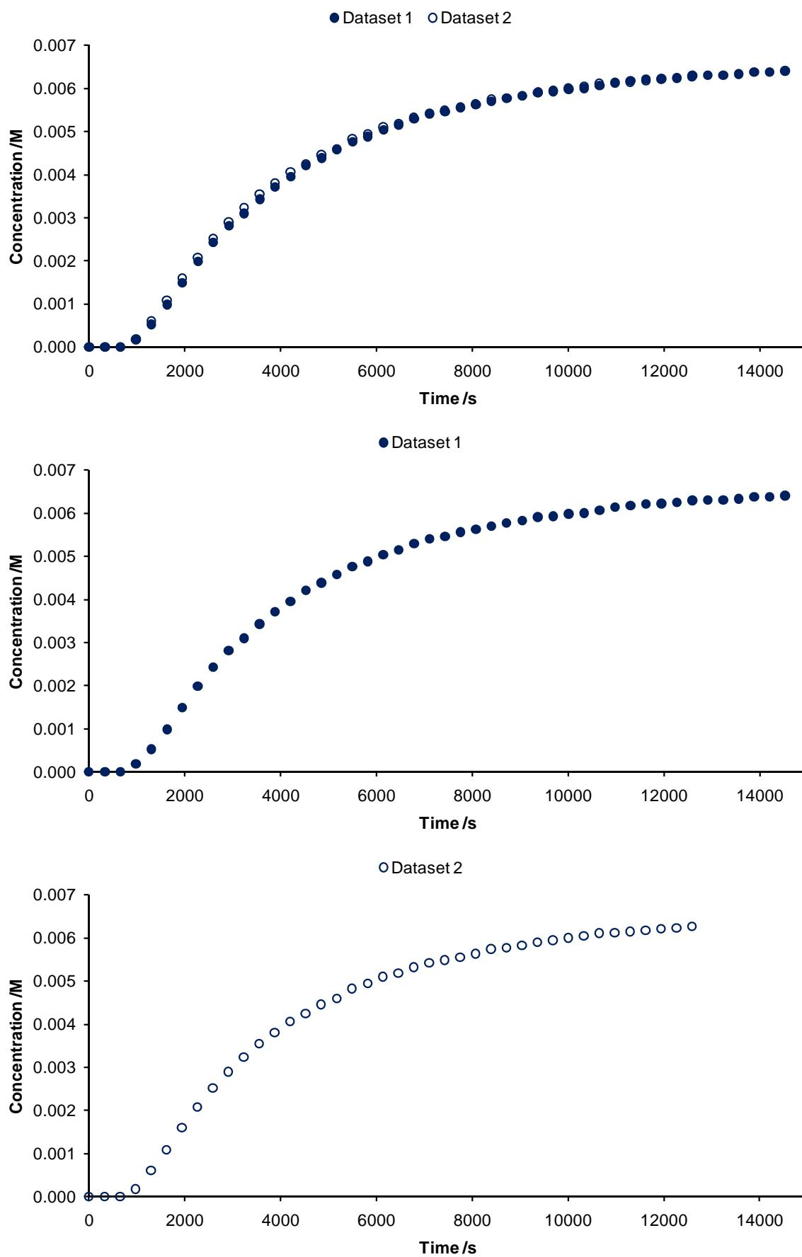
*Concentration/time data for the RCM of nonadiene **7d** with pre-catalyst **9** in CD<sub>2</sub>Cl<sub>2</sub> at 298 K (AV600, BBO-z-ATMA probe); 4 scans with D<sub>I</sub> = 35 s; TE = 298 K; concentrations obtained by integration of the appropriate signal and the internal standard (see above).*
