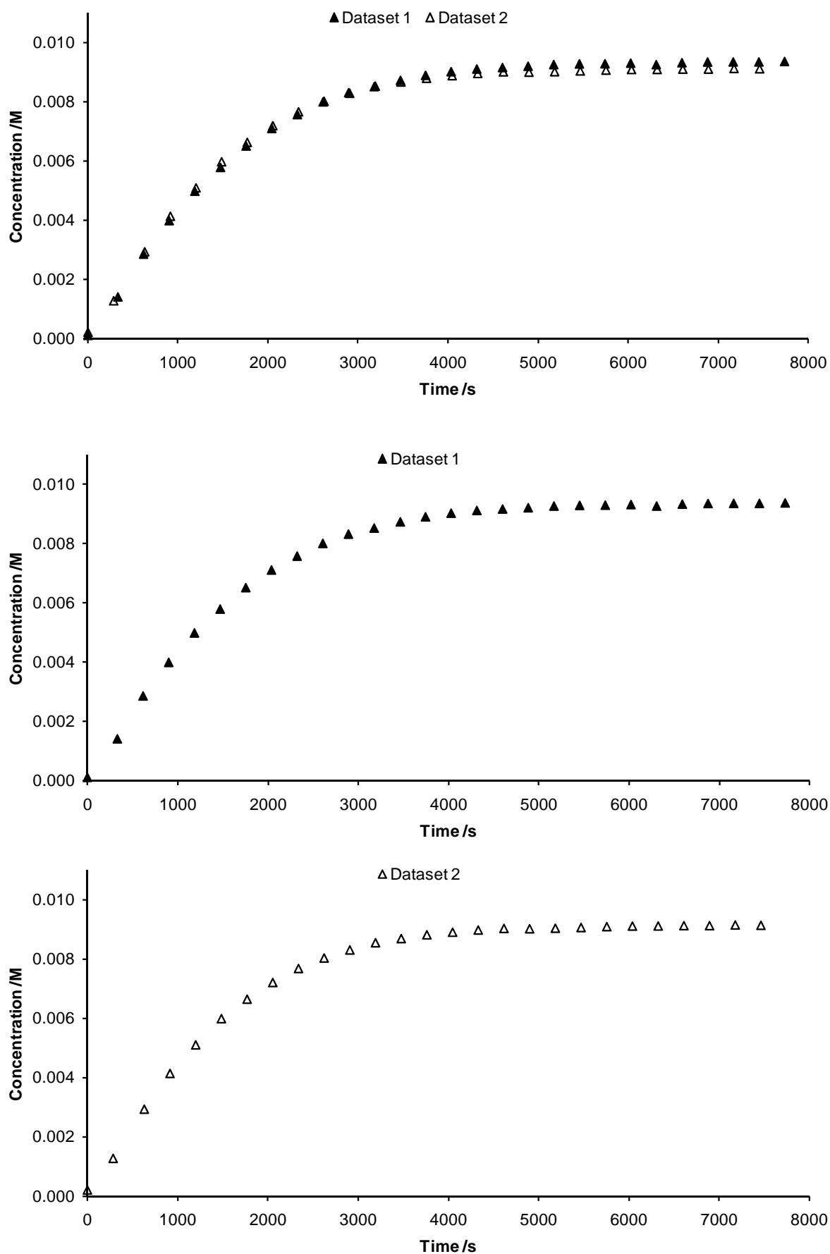
*Concentration/time data for the RCM of octadiene **7c** with pre-catalyst **9** in CDCl<sub>3</sub> at 298 K (AV400, BBFO-z-ATMA probe); 4 scans with D<sub>I</sub> = 35 s; TE = 298 K; concentrations obtained by integration of the appropriate signal and the internal standard (see above).*
