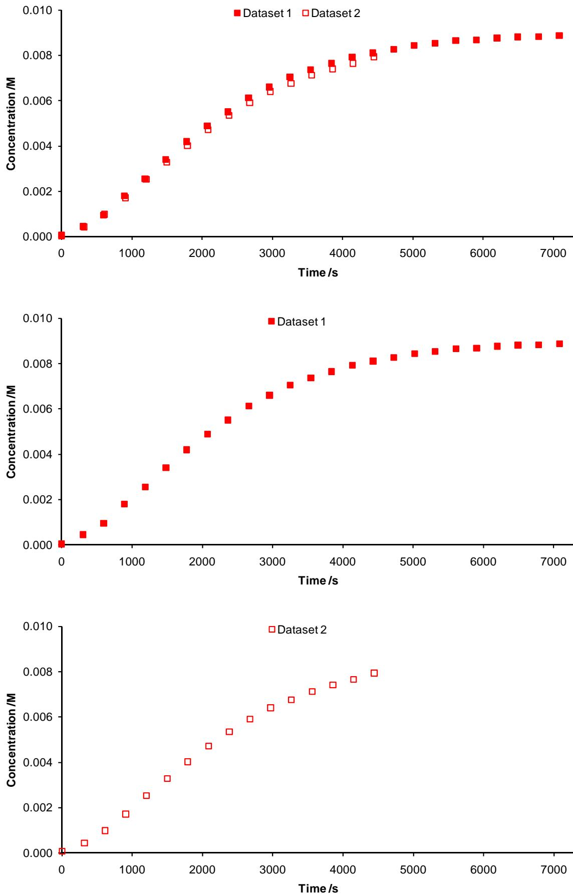
*Concentration/time data for the RCM of heptadiene **7b** with pre-catalyst **9** in  $CDCl_3$  at 298 K (AV400, BBFO-z-ATMA probe); 4 scans with  $D_I = 35$  s; TE = 298 K; concentrations obtained by integration of the appropriate signal and the internal standard (see above).*
