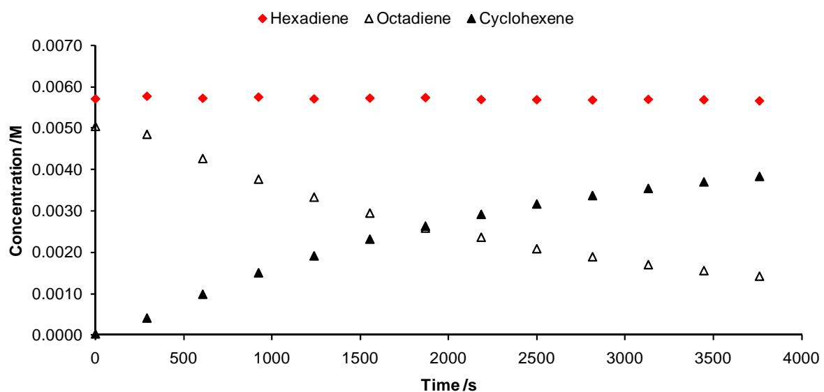
*Concentration/time data for the RCM of octadiene **7c** with pre-catalyst **9** in the presence of hexadiene **7a**, in CDCl<sub>3</sub> at 298 K (AV400, BBFO-z-ATMA probe); 4 scans with D<sub>I</sub> = 35 s; TE = 298 K; concentrations obtained by integration of the appropriate signal and the internal standard (see above).*
