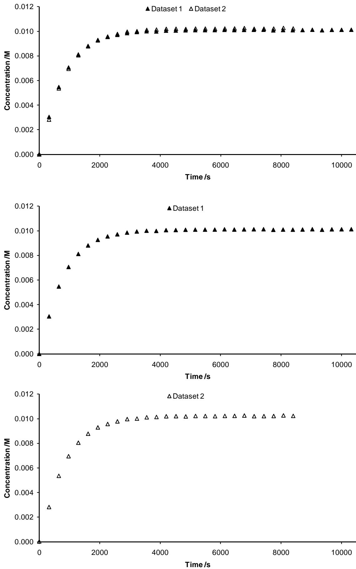
*Concentration/time data for the RCM of octadiene **7c** with pre-catalyst **9** in CD<sub>2</sub>Cl<sub>2</sub> at 298 K (AV600, BBO-z-ATMA probe); 4 scans with D<sub>I</sub> = 35 s; TE = 298 K; concentrations obtained by integration of the appropriate signal and the internal standard (see above).*
