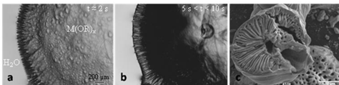
Figure 3: (a) Optical microscopy showing the accumulation of alcohol/water byproduct in the center of the alkoxide droplet as the reaction progresses (a,b) and corresponding SEM image (c).
