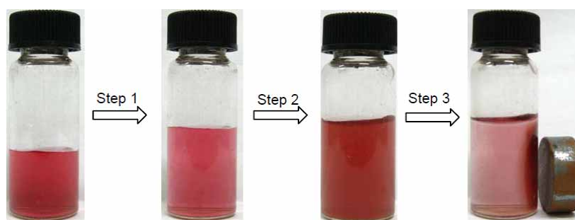
Fig. S8 The photos of overall process of DEA-Au NPs/ \text{Co}^{2+} absorbed by \text{Fe}_3\text{O}_4 nanoparticles in turn: well-dispersed DEA-Au NPs, addition of \text{Co}^{2+} , then addition of MA- \text{Fe}_3\text{O}_4 , and portion of Au NPs and \text{Fe}_3\text{O}_4 were attracted toward the magnet when a permanent magnet was set beside the bottle (the fourth photo). The process of DEA-Au NPs/M ( \text{M}=\text{Ag}^+ , \text{Mn}^{2+} , \text{Cd}^{2+} , \text{Ni}^{2+} , \text{Cu}^{2+} , \text{Hg}^{2+} , \text{Zn}^{2+} , \text{Fe}^{3+} , \text{Au}^{3+} ) absorbed by \text{Fe}_3\text{O}_4 is similar to DEA-Au NPs/ \text{Co}^{2+} .
