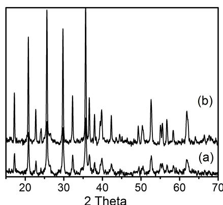
Figure S7. XRD patterns of  $\text{LiFePO}_4$  (a) after ball milling carbon coating, (b) after heat treatment at 600°C, under Ar and H<sub>2</sub> atmosphere for 4hours.
