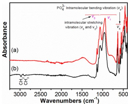
Figure S4. FTIR Spectra of LiFePO<sub>4</sub> nanocrystals synthesized in the (a) absence of oleylamine, (b) presence of oleylamine as capping and reducing agent.
