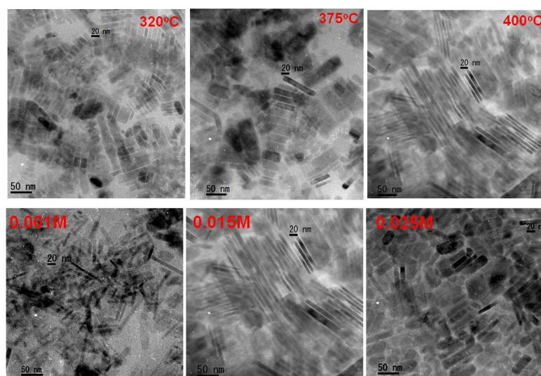
Figure S1. TEM images of LiFePO<sub>4</sub> nanocrystals synthesized at different temperature keeping constant precursor concentration 0.015M and at 10 min reaction time (top set). The bottom set images shows the nanocrystals formed at different precursor concentrations keeping reaction at constant reaction temperature 400°C for 10 min.
