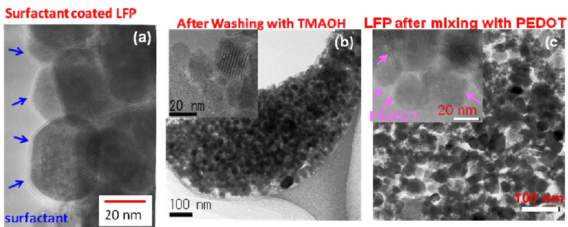
Figure S6. TEM image of (a) surface modified  $\text{LiFePO}_4$  nanocrystals, (b) after removal of surfactant by washing with tetramethylammonium hydroxide, (c)  $\text{LiFePO}_4$  nanocrystals surface coated PEDOT.
