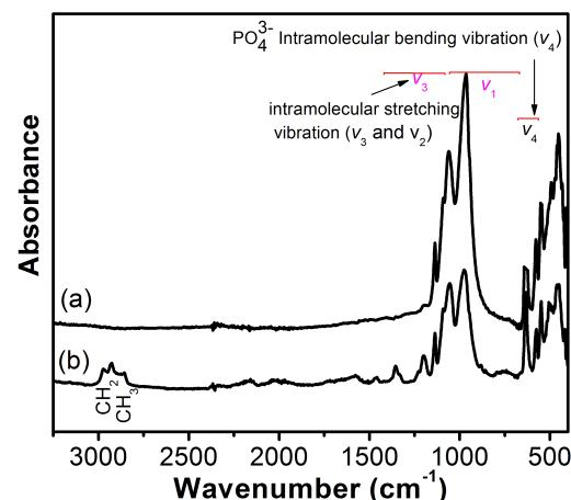
Figure S5. FTIR Spectra of LiMnPO<sub>4</sub> nanocrystals synthesized in the (a) absence of oleylamine, (b) presence of oleylamine as capping and reducing agent.
