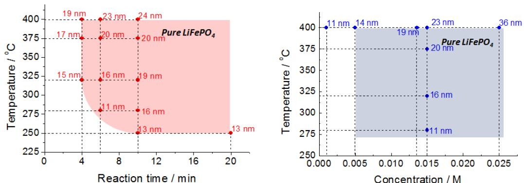
Figure S2. Effect of different reaction temperature and time/ precursor concentration on the particle size of the LiFePO<sub>4</sub> nanocrystals.
