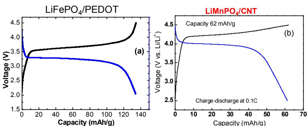
Figure S9. Charge-discharge profile of (a) LiFePO<sub>4</sub>/PEDOT nanoelectrode prepared without any additional heat treatment, (b) the LiMnPO<sub>4</sub>/CNT nanocrystals electrode prepared with carbon coating under ball milling followed by heat treatment at 600°C, under Ar and H<sub>2</sub> atmosphere for 4 h. The current density for charge-discharge measurement was 0.1C.
