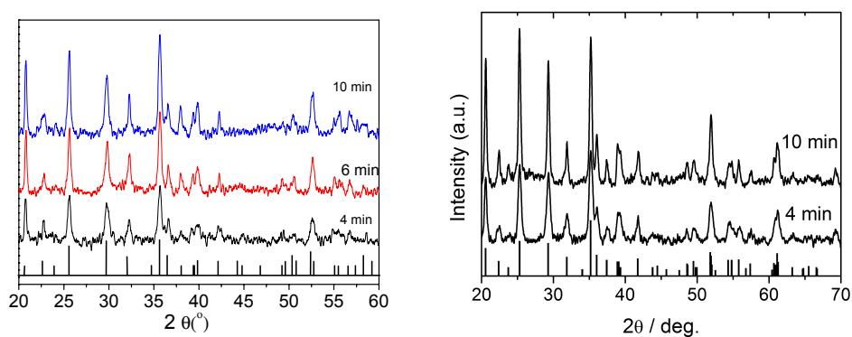
Figure S3 XRD patterns of the LiFePO<sub>4</sub> (left hand side) and LiMnPO<sub>4</sub> (right hand side) nanocrystals synthesized at different reaction time and at 400 °C.
