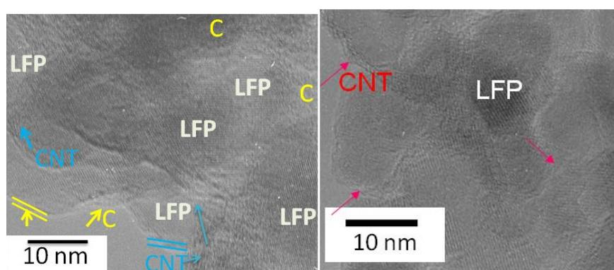
Figure S8. HR-TEM images of  $\text{LiFePO}_4$  after ball milling carbon coating and heat treatment.
