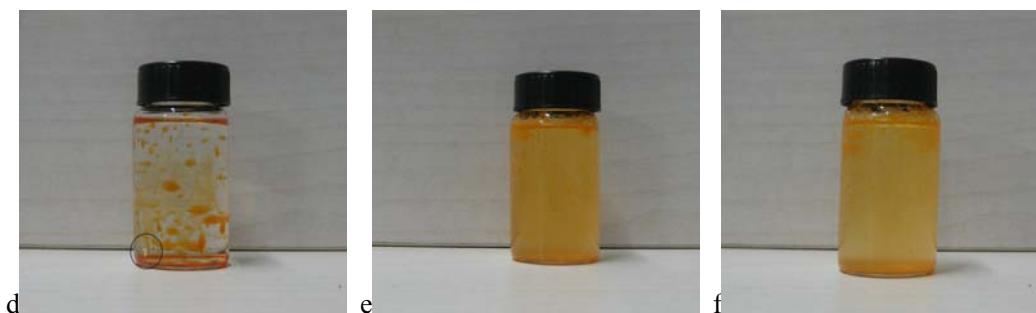
Figure S4. Optical images of hexane/water system without and with PS/P4VP particles: a) methyl orange aqueous added into hexane, b) the system under ultrasonication, c) the system standing for 5 minutes; d) PS/P4VP composite particles added into the hexane/water system, e) the system under ultrasonication, f) the system standing for 30 minutes.
