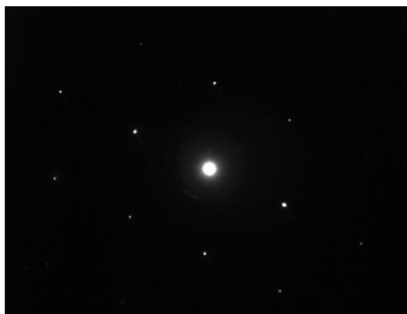
Figure S3. The reciprocal lattice peaks, which were obtained from 2D Fourier transform of the lattice resolved TEM image for the hydrogenated graphene sample
