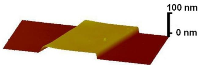
Fig. S2. AFM image of the  $\text{Co}_2\text{Si}$  nanobelt used in electrical and MR measurements shows an overall thickness of 25 nm (including surface oxide layers). The image area is  $2 \mu\text{m} \times 1 \mu\text{m}$ .
