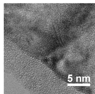
Fig. S3: TEM image of  $\text{Co}_2\text{Si}$  nanobelt with 7 nm silicon oxide shell.
