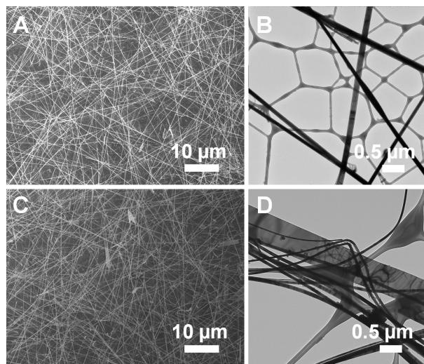
Fig. S1. SEM and TEM images of the nanostructures obtained at various temperatures of  $\text{CoCl}_2$  precursor: (A), (B) 600 °C; (C), (D) 615 °C.
