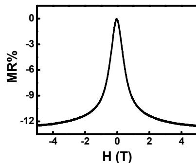
Fig. S4. Magnetoresistance curve of the  $\text{Co}_2\text{Si}$  nanobelt in the range of  $\pm 5 \text{ T}$  at 1.5 K.
