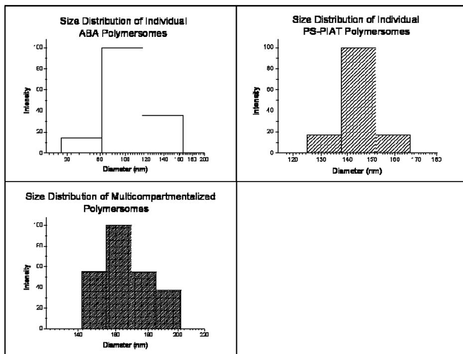
**Figure S1.** DLS data showing the distinctly different sizes of the polymersomes. There is a clear increase in sizes, with individual ABA polymersomes having the smallest diameter (average 100 nm) and the multicompartimentalized polymersomes having the largest (average 160 nm).
