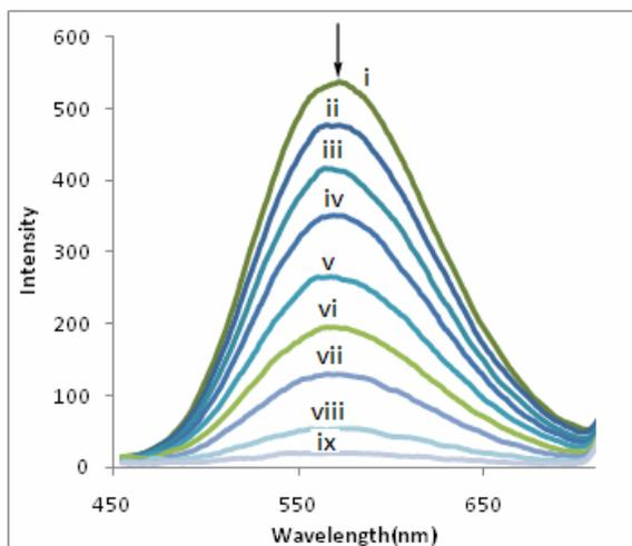
**Figure S11:** Fluorescence responses in aqueous solution buffered at pH 7.2 of (i) the free  $L_2$  and of that after addition of (ii) 0.1 equivalent, (iii) 0.3 equivalent, (iv) 0.4 equivalent, (v) 0.5 equivalent, (vi) 0.6 equivalent, (vii) 0.7 equivalent, (viii) 0.9 equivalent and (ix) 1.0 equivalent of  $[\text{Cu}(\text{H}_2\text{O})_6]^{2+}$ .
