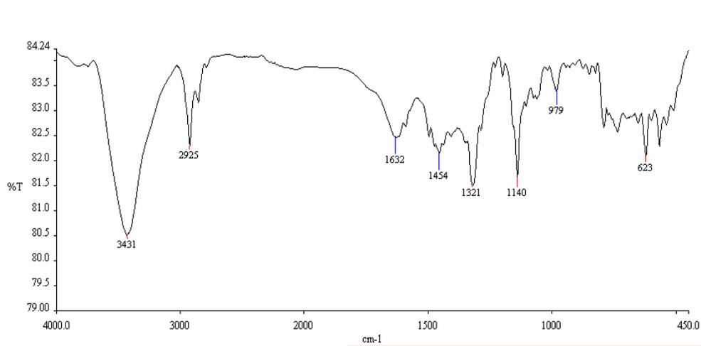
**Figure S4:** FT-IR spectrum of L<sub>2</sub> in KBr pellet.
