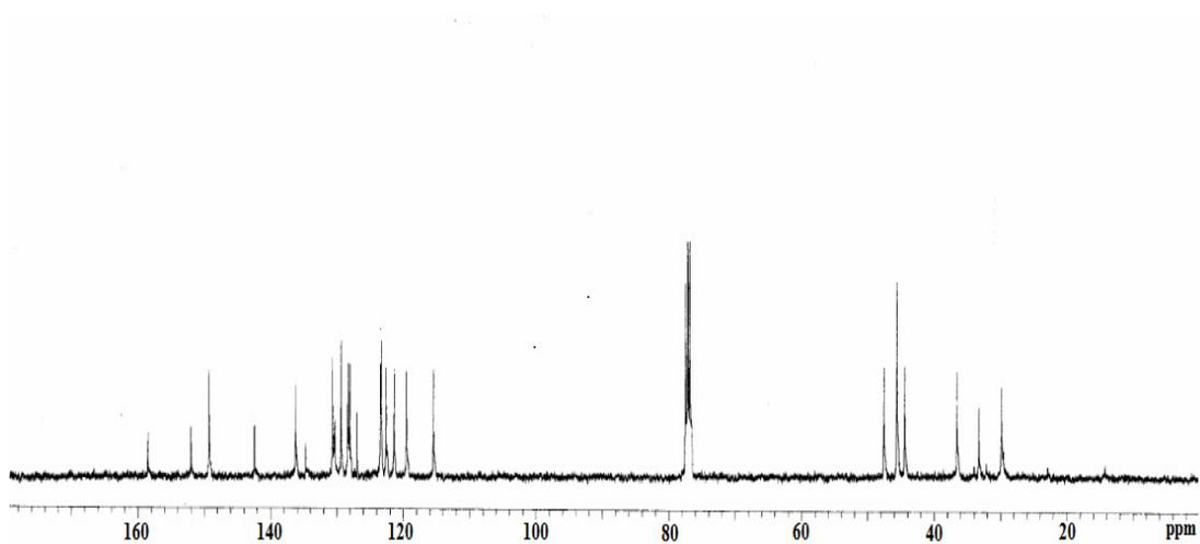
**Figure S6:** <sup>13</sup>C-NMR spectrum of the L<sub>2</sub> in CDCl<sub>3</sub>.
