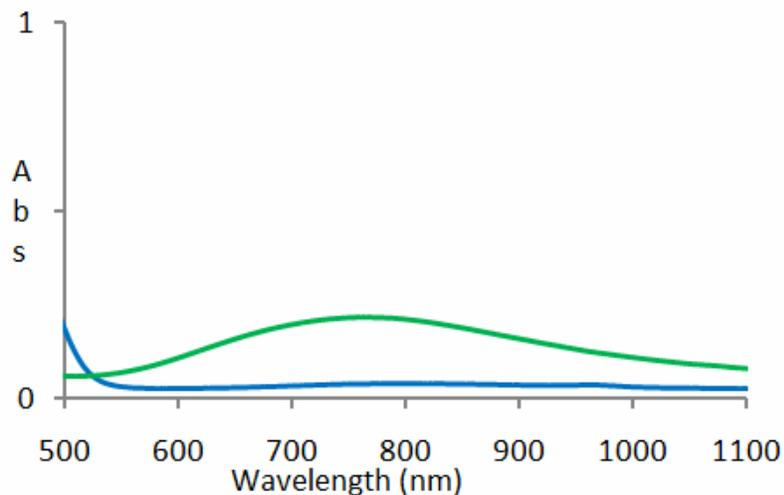
**Figure S13:** UV-visible spectra of complex **1** before (green line) and after (blue line) purging nitric oxide in aqueous medium buffered at pH 7.2.
