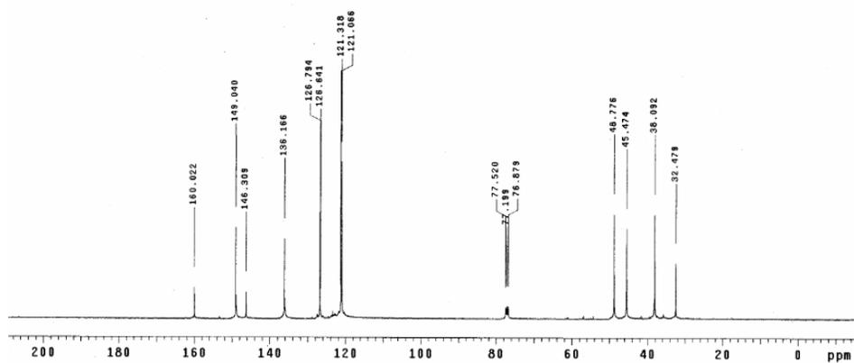
**Figure S3:** <sup>13</sup>C-NMR spectrum of L<sub>1</sub> in CDCl<sub>3</sub>.
