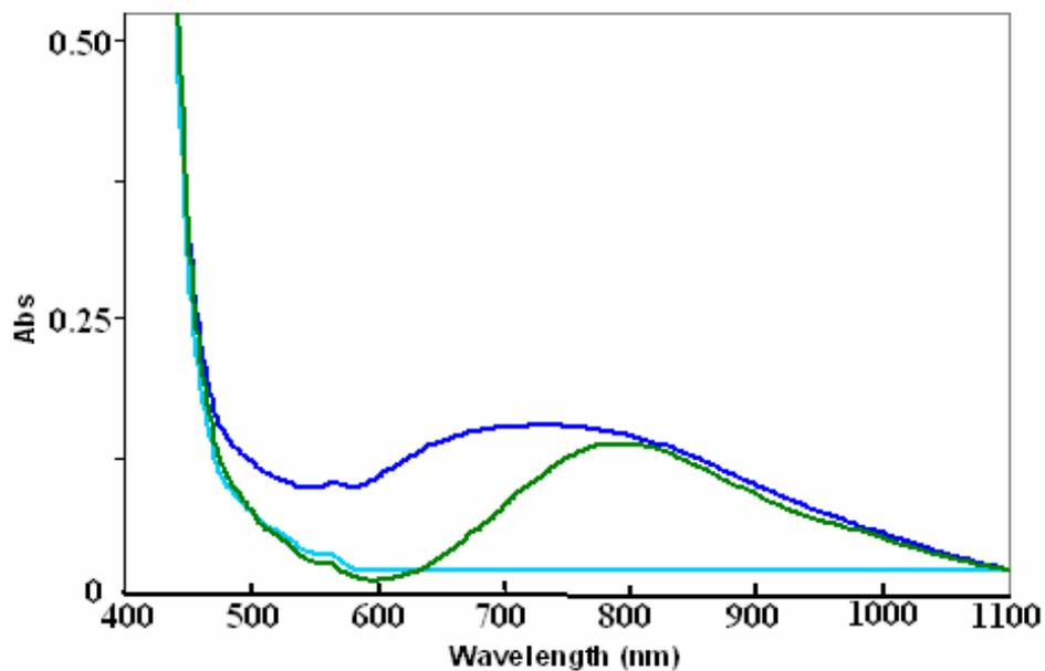
**Figure S16:** UV-visible spectra of complex **1** (dark blue), immediately after its reaction with NO (light blue) in methanol. The green trace is that of the solution obtained after keeping the reduced species for 2 h at open air and at room temperature.
