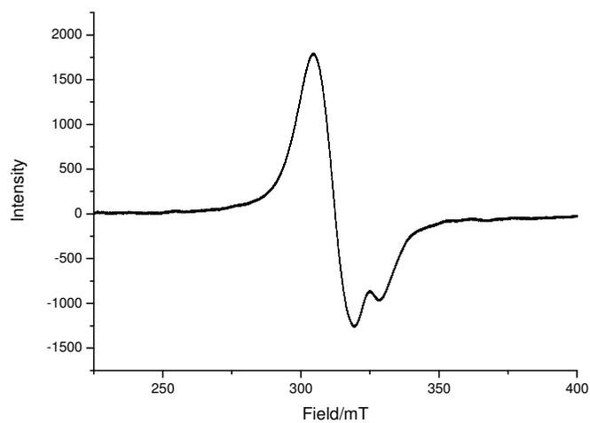
**Figure S9:** X-band EPR spectrum of complex **1** in MeOH at room temperature.
