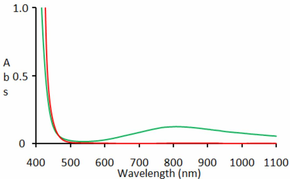
**Figure S14.** UV-visible spectra of complex **1**(green line) and after its reaction with NO (red line) in methanol solution.
