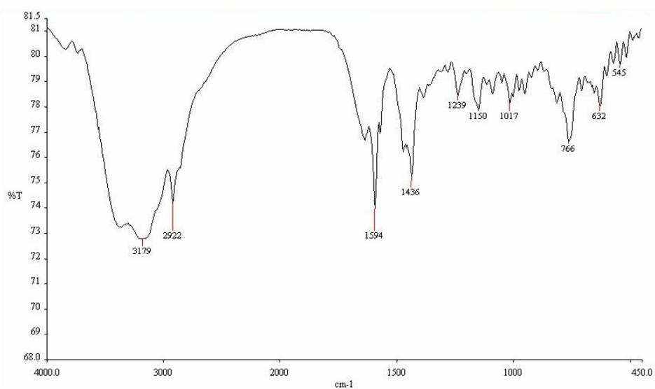
**Figure S1:** FT-IR spectrum of L<sub>1</sub> in KBr pellet.
