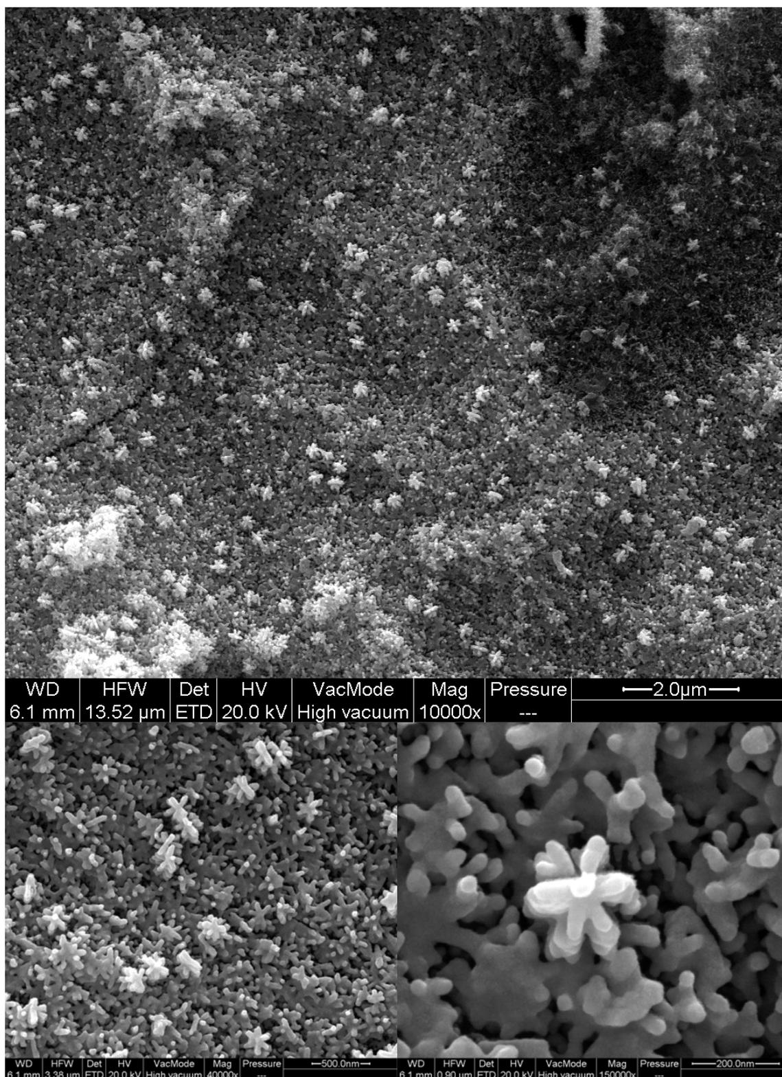
**Figure S2** SEM images with different magnifications of R-TiO<sub>2</sub> nanostructures grown under 8 M HCl. The nanoflowers are obviously not densely populated as compared to that obtained under 6 M HCl.
