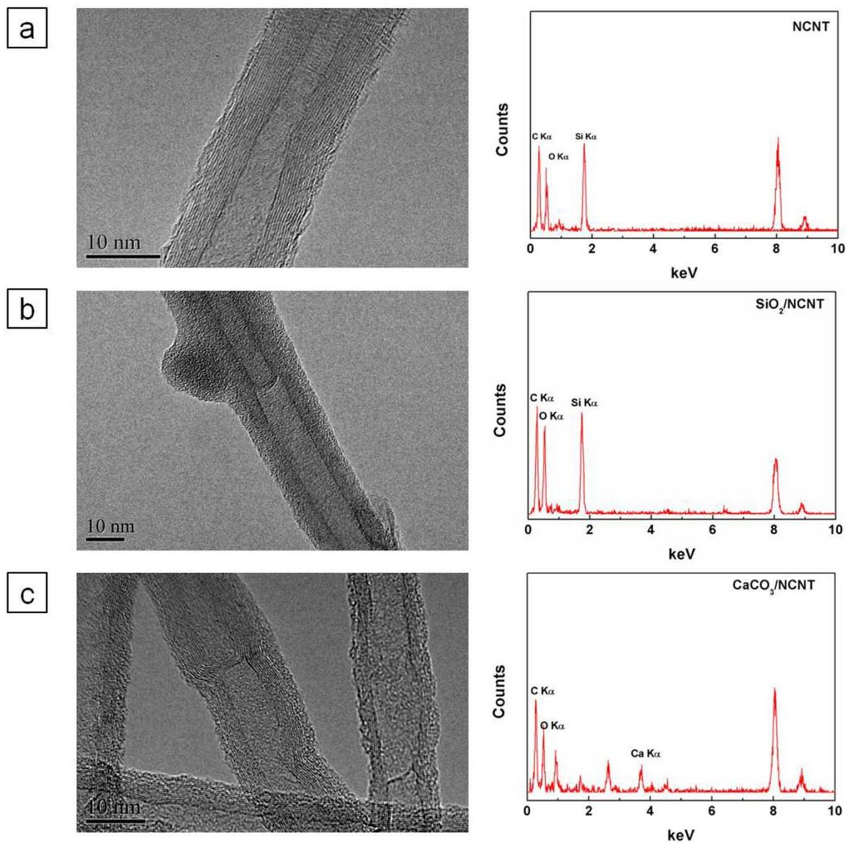
**Fig. S1** TEM images and EDX chemical analyses of (a) bare NCNTs, (b) SiO<sub>2</sub> coated NCNTs, and (c) CaCO<sub>3</sub> coated NCNTs.
