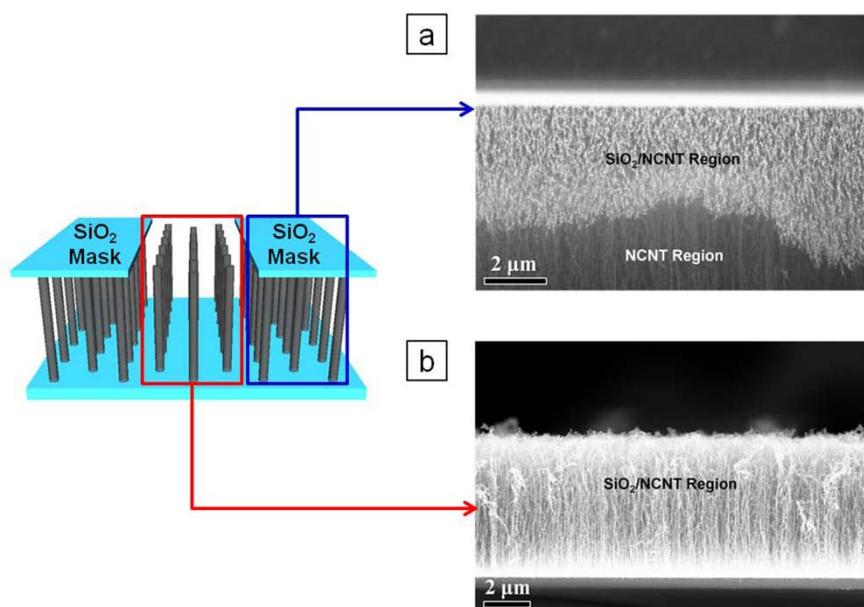
**Fig. S5** Comparison between (a) SiO<sub>2</sub> half coated NCNTs and (b) SiO<sub>2</sub> fully coated NCNTs.
