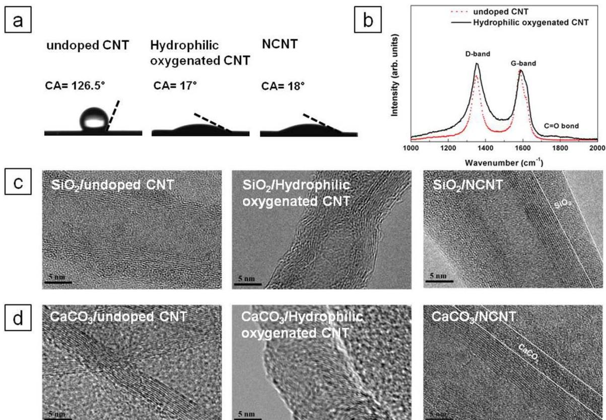
**Fig. S3** (a) Static water contact angles (CA) of undoped CNT, hydrophilic oxygenated CNT, and NCNT, (b) FT-Raman spectrum of undoped CNT and hydrophilic oxygenated CNT, TEM images of (c) SiO<sub>2</sub>/undoped CNT (left), SiO<sub>2</sub>/hydrophilic oxygenated CNT (middle), and SiO<sub>2</sub>/NCNT (right), (d) CaCO<sub>3</sub>/undoped CNT (left), CaCO<sub>3</sub>/hydrophilic oxygenated CNT (middle), and CaCO<sub>3</sub>/NCNT (right).
