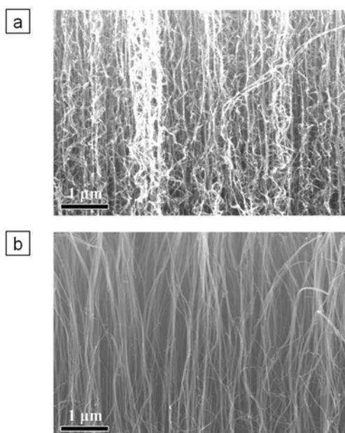
**Fig. S4** Individually separated (a) SiO<sub>2</sub> coated NCNTs and (b) CaCO<sub>3</sub> coated NCNTs.
