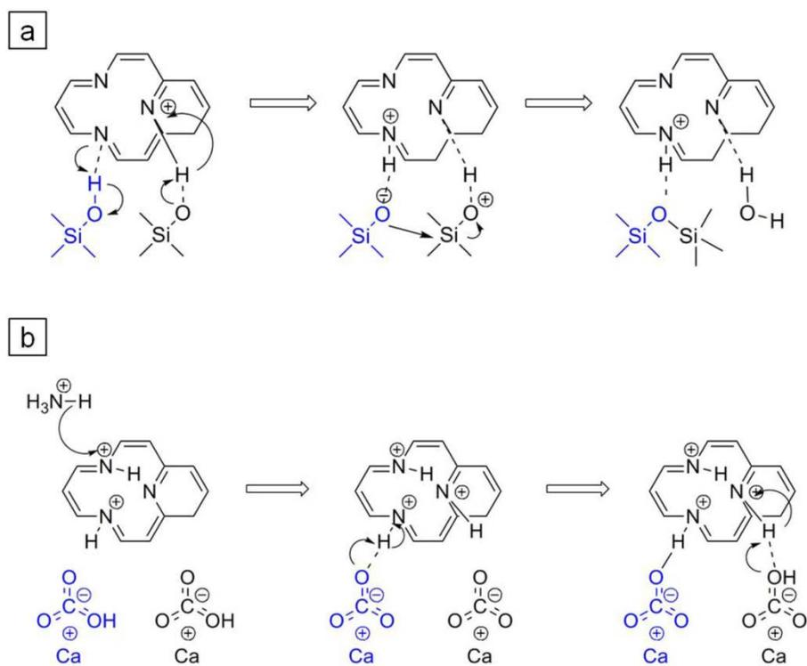
**Fig. S6** Proposed biomimetic mineralization mechanisms for (a) SiO<sub>2</sub> coated NCNTs, and (b) CaCO<sub>3</sub> coated NCNTs at pyridinic nitrogen nucleation sites.
