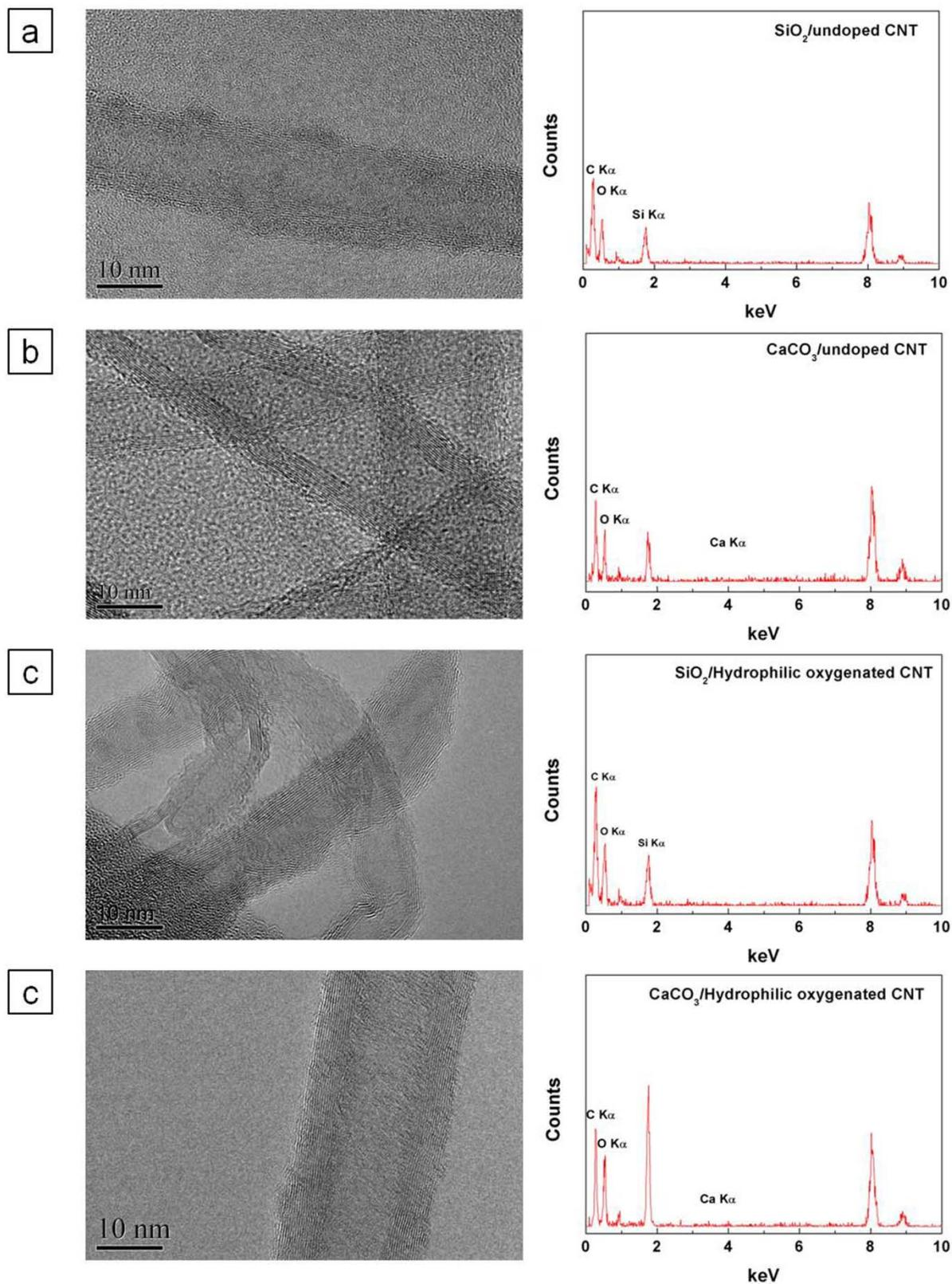
**Fig. S2** TEM images and EDX chemical analyses of (a) SiO<sub>2</sub>/undoped CNT, (b) CaCO<sub>3</sub>/undoped CNT, (c) SiO<sub>2</sub>/Hydrophilic oxygenated CNT, and (d) CaCO<sub>3</sub> / Hydrophilic oxygenated CNT.
