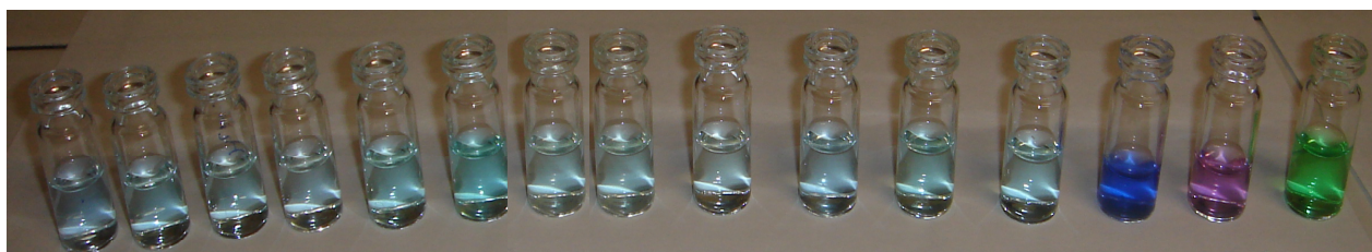
Figure S5. Colour change of 1 ( 1.00 \times 10^{-3} M) after addition of different anions in MeCN. From left to right: 1 , 1 + 1 eq. of F - , 1 + 1 eq. of Cl - , 1 + 1 eq. of Br - , 1 + 1 eq. of MeCO 2 - , 1 + 1 eq. of PhCO 2 - , 1 + 1 eq. of H 2 PO 4 - , 1 + 1 eq. of HSO 4 - , 1 + 1 eq. of HCO 3 - , 1 + 1 eq. of NO 3 - , 1 + 1 eq. of N 3 - , 1 + 1 eq. of SCN - , 1 + 1 eq. of CN - , 1 + 2 eqs. of CN - , 1 + 1 eq. of I - .
