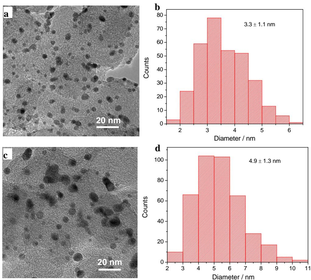
**Fig. S2** TEM images and histogram of particle sizes of Pt/C catalyst before (a, b) and after (c, d) the durability test of 20,000 potential cycles. After the stability test, the average particle size of Pt/C significantly increases from 3.3 to 4.9 nm.
