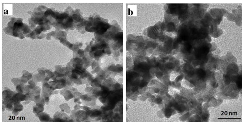
Fig. S3. TEM images of Pt black catalysts before (a) and after (b) the durability test of 20,000 potential cycles. After the stability test, the degree of agglomeration becomes greater.
