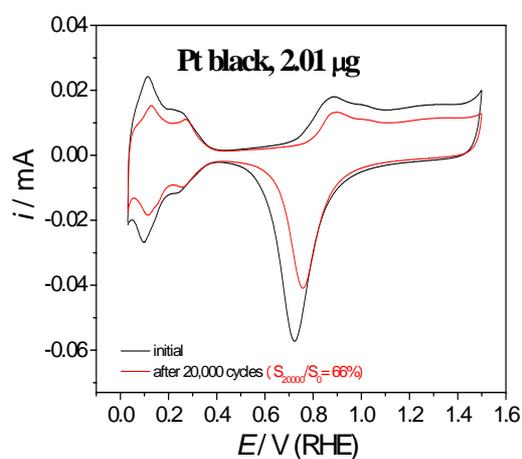
**Fig. S1** The electrochemical durability of commercial Pt black with lower loading (2.01 μg). Other conditions are same with those in Fig. 3b.
