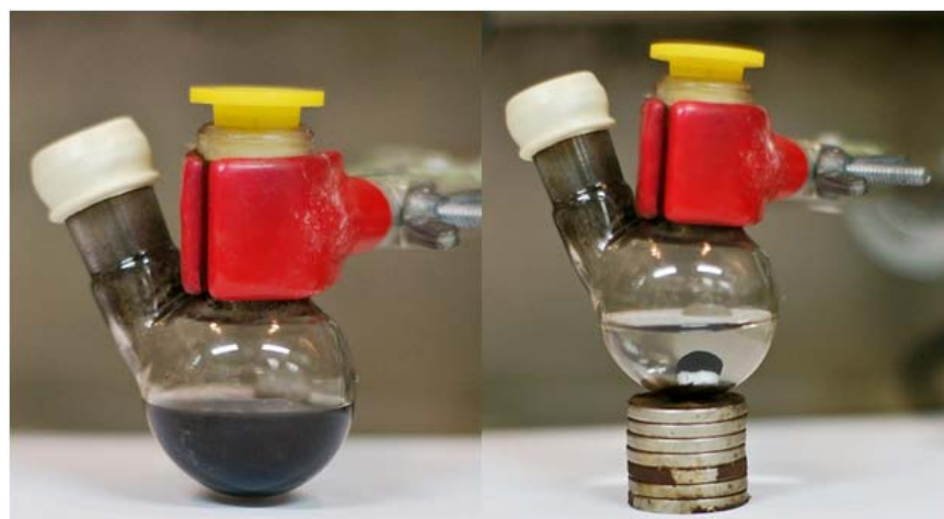
Figure S4. Photographs showing the magnetic separation of the catalysts in the mixture solution after the catalytic reaction.
