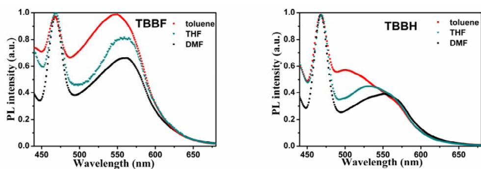
**Fig. S5** Emission spectra of **TBBF** (left) and **TBBH** (right) in toluene, **THF**, **DMF**.
