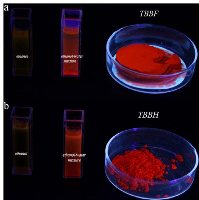
**Fig. S1** (a) The fluorescence of **TBBF** in ethanol (left), ethanol/water = 1:9 (middle) and solid of **TBBF** under illumination with a 365.0nm lamp (right). (b) The fluorescence of **TBBH** in ethanol (left), ethanol/water = 1:9 (middle) and solid of **TBBH** under illumination with a 365.0nm lamp (right).
