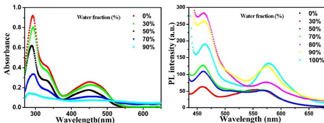
**Fig. S2** Absorption and **PL** spectra of **TBBH** in ethanol-water mixtures with different fractions of water;  $c = 5\mu\text{M}$ .
