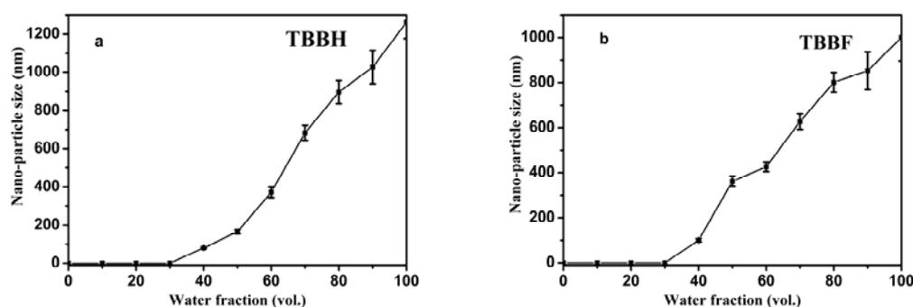
**Fig. S4** The nano-particle size of **TBBH** (a) and **TBBF** (b) in ethanol/water solution.
