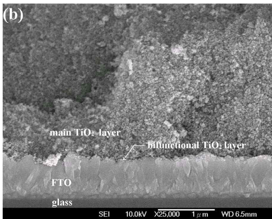
Fig. S3 Cross-sectional micrographs of photoanodes employing (a) FTO substrate and (b) TiO 2 -coated FTO substrate.
