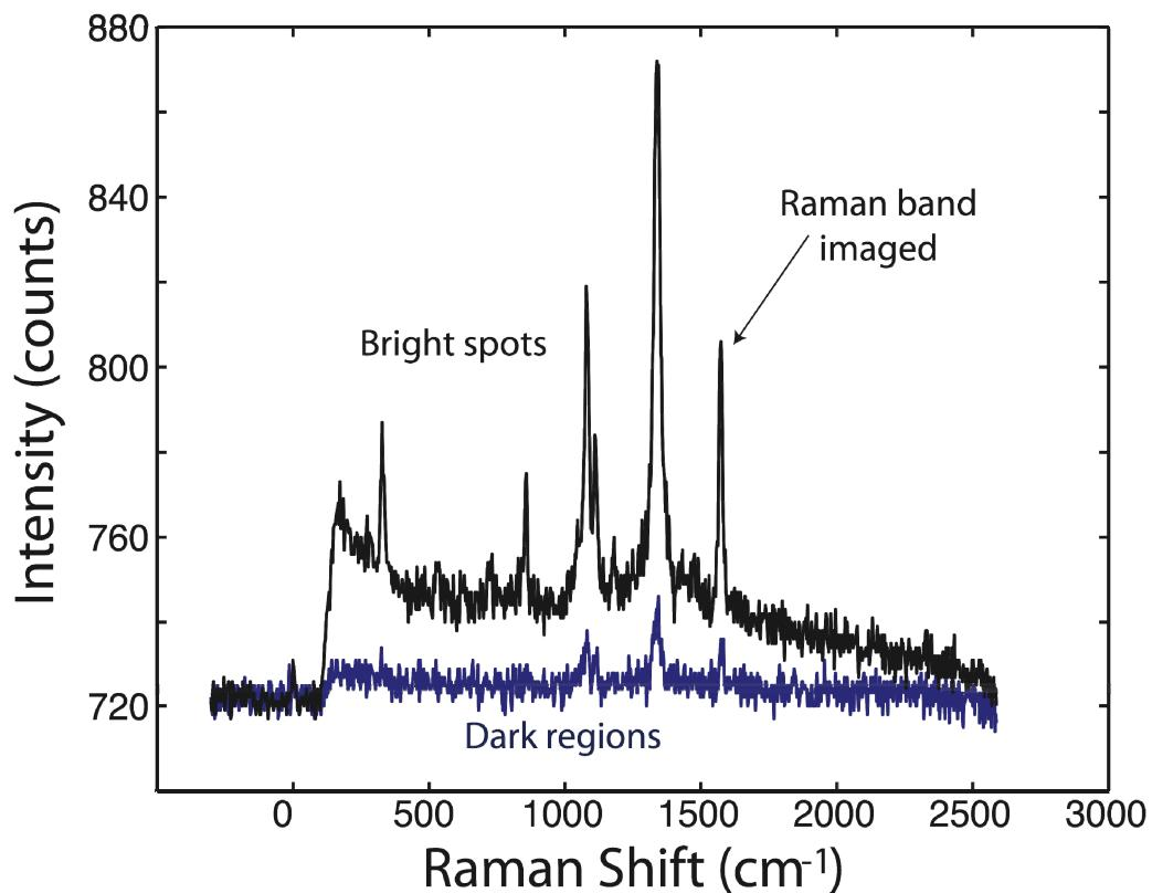
Figure S1. SERS spectra of 4-nitrobenzenethiol on the nanostructured surfaces. The spectrum in black corresponds to the bright regions of the Raman images, while the spectrum in blue corresponds to the dark regions of low SERS intensity. The 4-NBT band at a  $1574\text{ cm}^{-1}$  was mapped in the Raman images.
