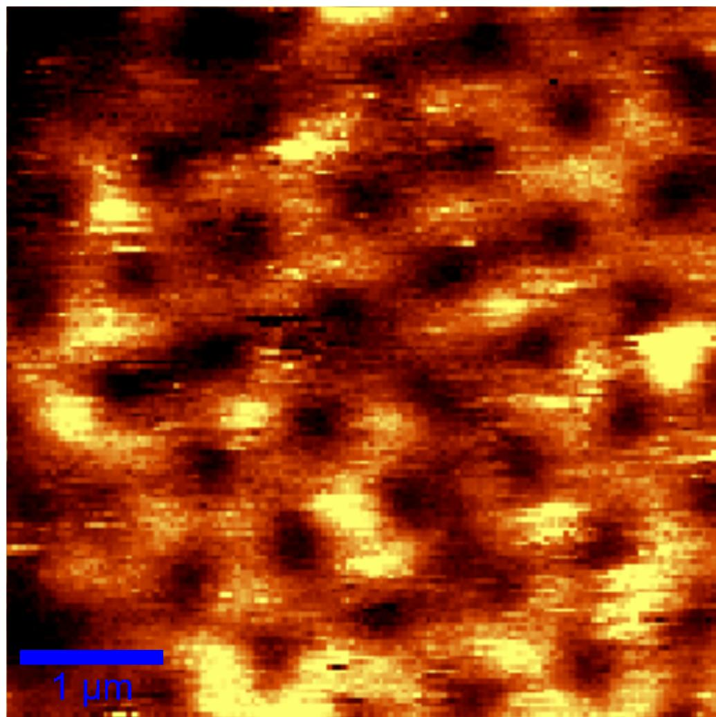
Figure S4. Raman image with high spatial resolution of D/P 0.69 with a scanning area of  $5 \times 5 \mu\text{m}$
