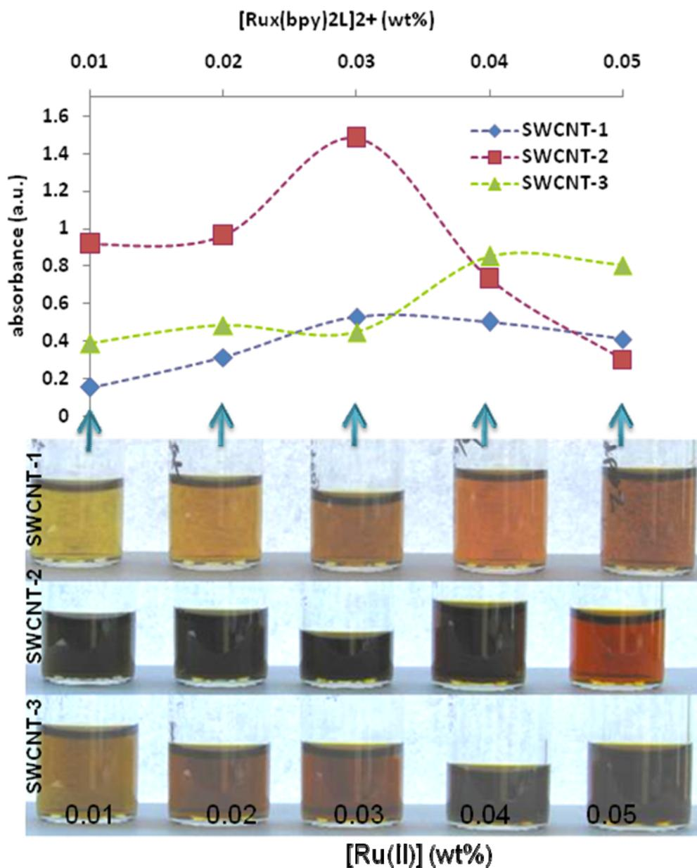
**Figure S2b: Photographs of (a)SWCNT-1, (b)SWCNT-2 and (c)SWCNT-3 solutions after centrifugation.**
