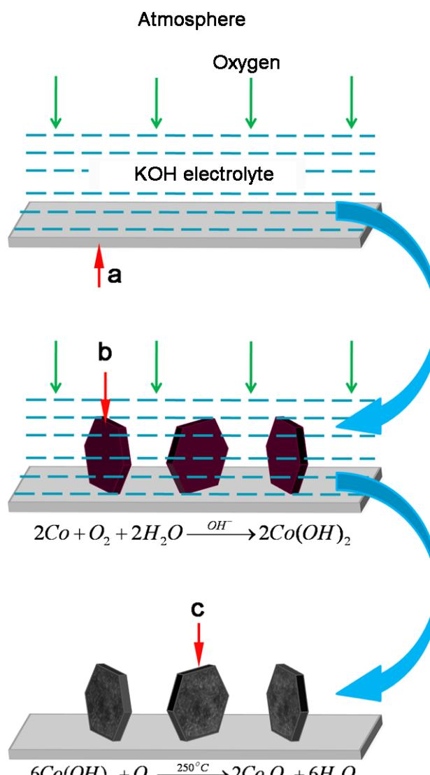
**Scheme S1** Synthesis of freestanding 2D  $\text{Co}_3\text{O}_4$  nanosheets. (a) Cobalt metal electrodeposited on conductive substrate; (b) Hexagonal brucite-like  $\beta\text{-Co}(\text{OH})_2$  precursor and (c) Freestanding  $\text{Co}_3\text{O}_4$  nanosheets.
