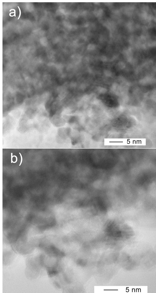
**Fig. S2** Close view TEM images of  $\text{Co}_3\text{O}_4$  nanosheets. The observed pore size was mainly less than 5 nm. The average  $\text{Co}_3\text{O}_4$  particle size was calculated by XRD pattern (figure 1) according to Scherrer equation:
