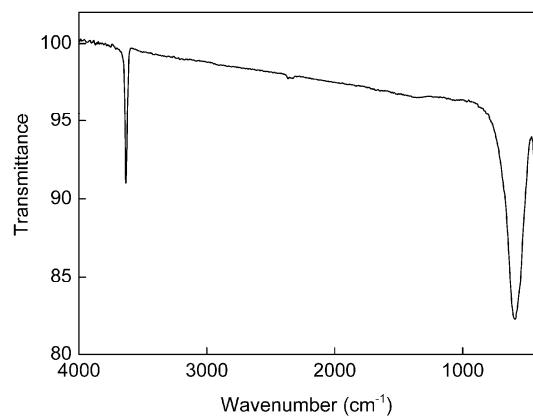
**Fig. S5** FT-IR spectra of the  $\beta\text{-Co(OH)}_2$  precursor. The sharp peak observed at 3630  $\text{cm}^{-1}$  is assigned to overlapping stretching modes of hydroxyl group in the brucite-like structure.<sup>3</sup> The peak at 590  $\text{cm}^{-1}$  is associated with Co-O stretching and Co-OH bending vibrations. The FT-IR spectra was determined on an Nicolet Nexus 470 FT-IR analyzer. A polished Cobalt plate was used as the background.
