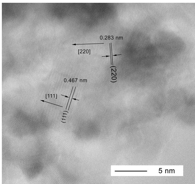
**Fig. S3** High resolution figure of HRTEM of  $\text{Co}_3\text{O}_4$  nanosheets. The high resolution transmission electron microscopy (HRTEM) image (Figure 3c) shows a well-defined crystalline structure with lattice spacing of 0.467 Å and 0.283 Å, corresponding to the value of the (111) and (220) plane of the  $\text{Co}_3\text{O}_4$  phase.
