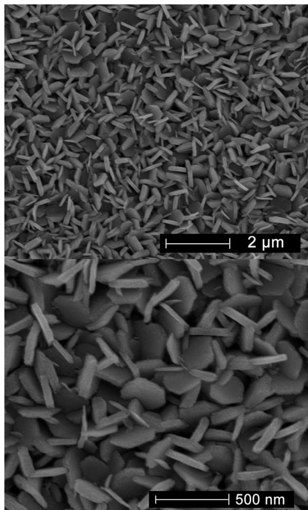
**Fig. S1** (a) SEM and (b) close view SEM images of  $\text{Co}_3\text{O}_4$  nanosheets coating with a conductive platinum layer.
