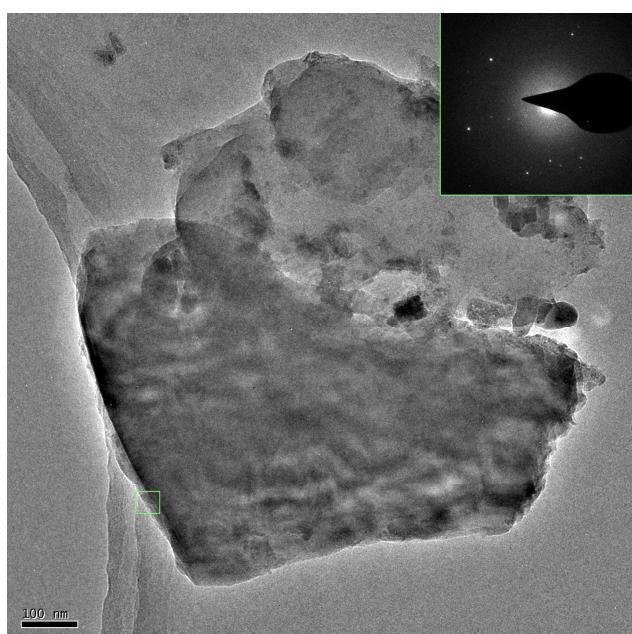
**Fig. S6** TEM image and selected-area electron diffraction (SAED) of cobalt hydroxide precursor.
