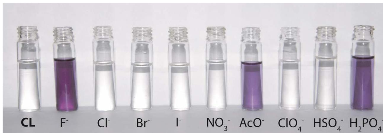
**Figure S27.** Colour changes observed with the addition of excess anions to acetonitrile solutions of **CL**.
