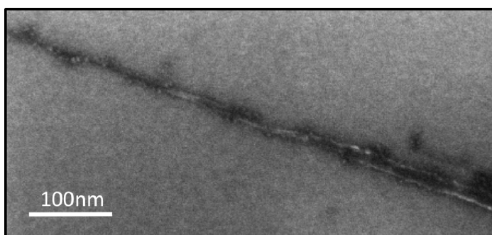
Fig. S4 A high-resolution scanning electron microscopy (SEM) image of Co oxide nanoparticles aligned along SWNTs. To obtain the maximum resolution, SWNT-protein complex in pure H 2 O was put onto a surface-cleaned silicon oxide substrate. Protein shell is not visible in SEM image.
