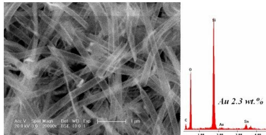
**Fig. S1.** SEM image of AuNPs/SNTs nanocomposite with well-dispersed distribution of small AuNPs using Backscattered electron (BSE) mode, and the corresponding EDX spectrum.
