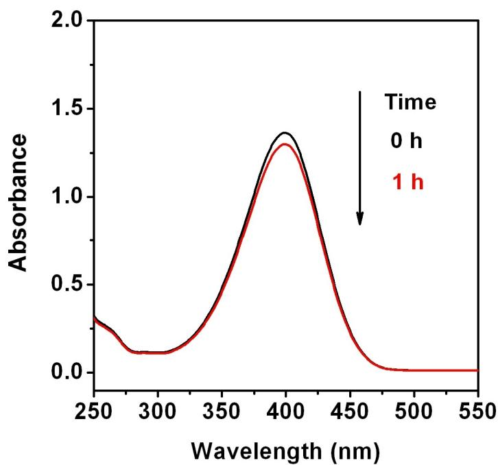
**Fig. S4.** UV-Vis absorption spectra of 4-NP in the presence of  $\text{Sn}^{2+}$  activated SNTs and  $\text{NaBH}_4$  for 1h.
