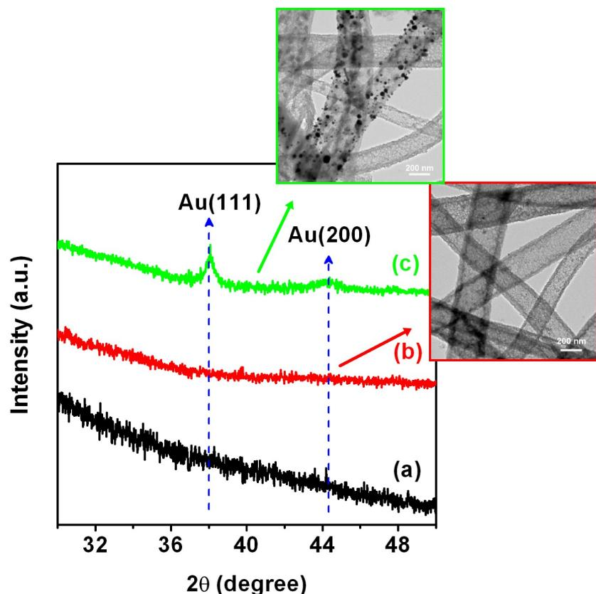
**Fig. S3.** XRD patterns and the corresponding TEM images of as-prepared products: (a) SNTs; (b) AuNPs/SNTs nanocomposite prepared by low concentration of HAuCl<sub>4</sub>; (c) AuNPs/SNTs nanocomposite prepared by high concentration of HAuCl<sub>4</sub>.
