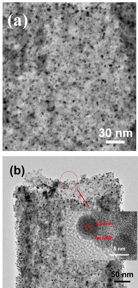
**Fig. S2.** (a) TEM image of well-dispersed AuNPs with the size of 3-5 nm on the surface of electrospun STs. (b) TEM image of AuNPs/SNTs nanocomposite; the insert was the HRTEM image of AuNP on the inside surface of electrospun SNTs.
