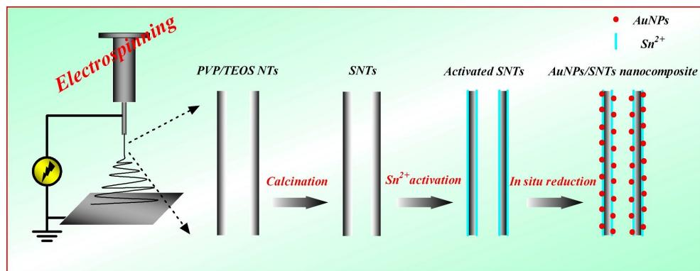
**Scheme 1.** Schematic diagram of the fabrication of AuNPs/SNTs nanocomposite.
