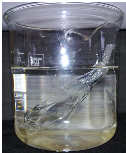
Figure 3S. Recyclability of catalyst 1b from aqueous reaction residue using a simple dialysis technique.
